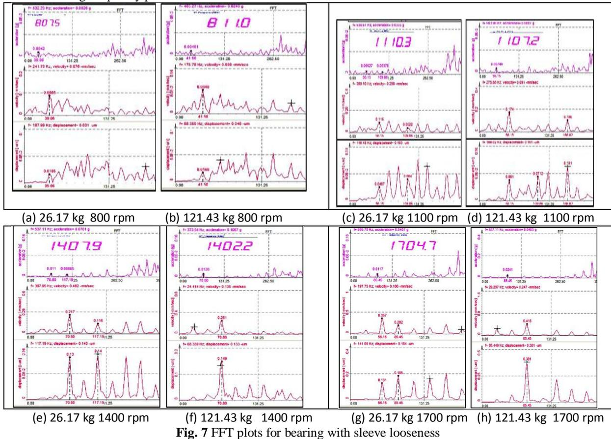
Fig. 7 FFT plots for bearing with sleeve looseness
