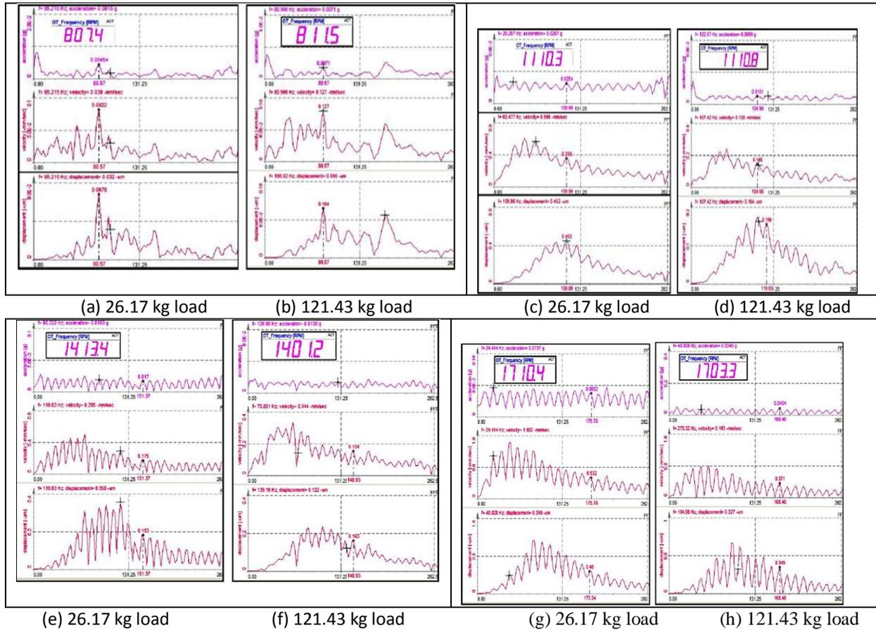
**Fig. 6** FFT plots for bearing with ball defect in all readings. The table 4 below shows the frequencies of predominant peak for speed steps.
