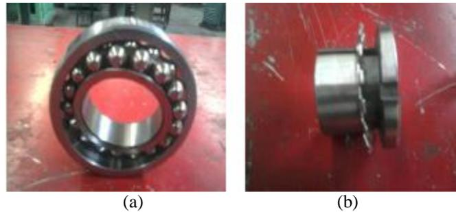
Fig.1 a) 1209 EKTN bearing and b) H209 Adapter sleeve
