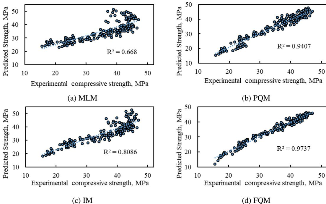
Fig.12 Experimental values versus predicted compressive strengths
