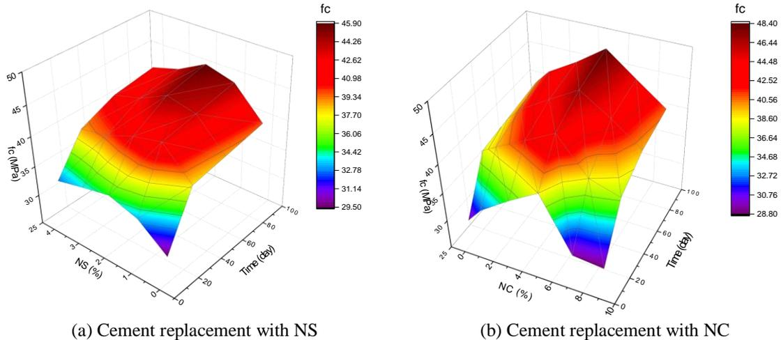
Fig.1 Compressive strengths (At ambient temperatures)
