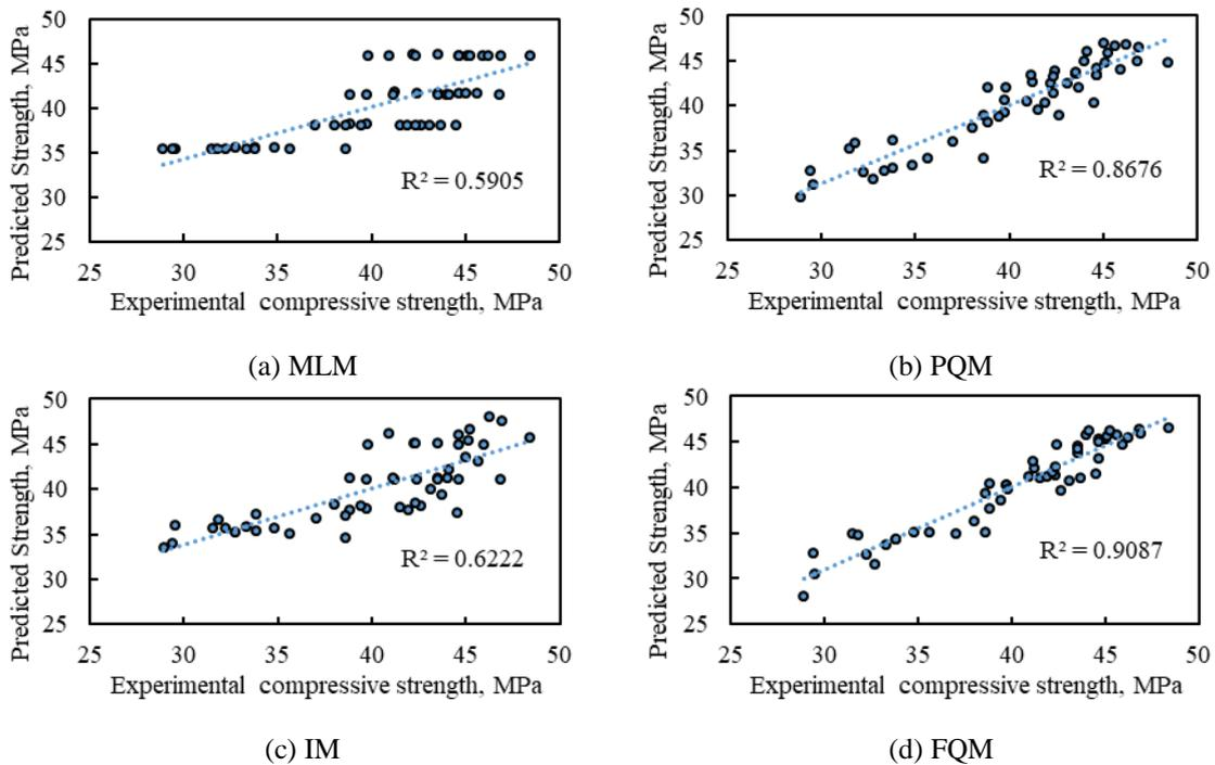
Fig.6 Experimental values versus predicted compressive strengths (At ambient temperature)
