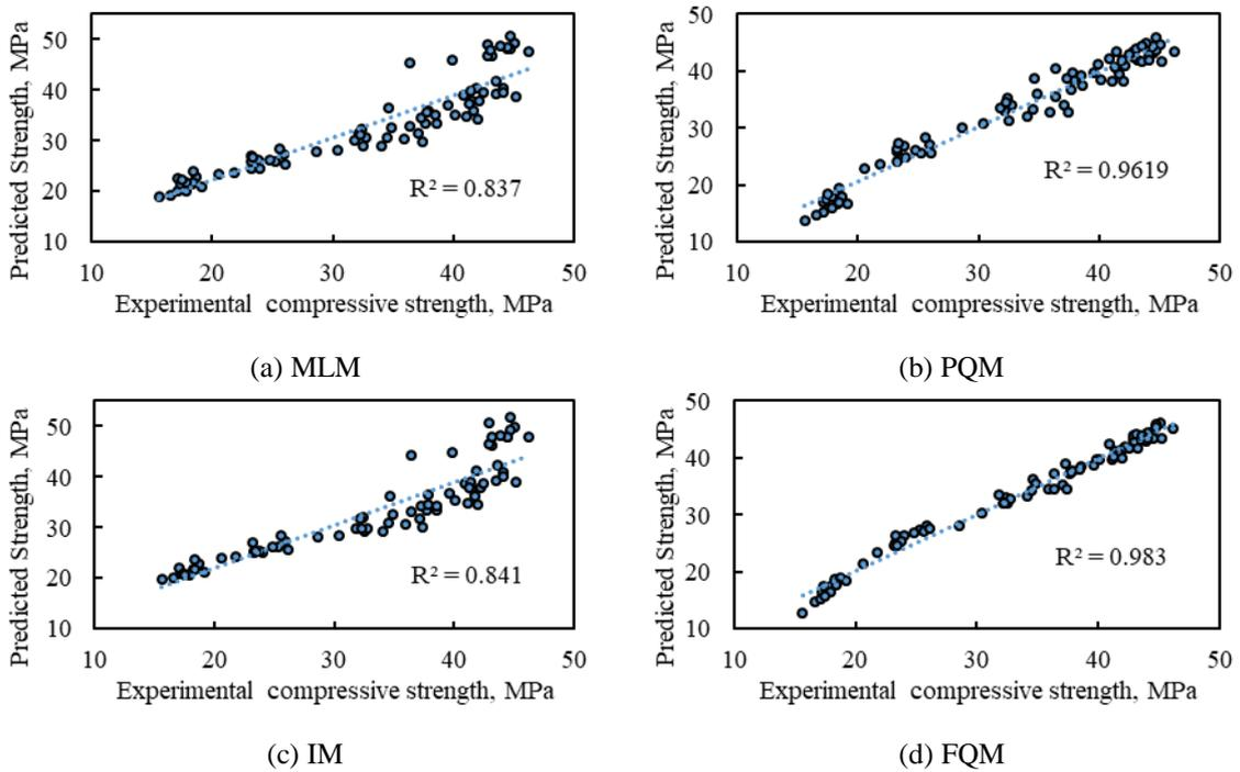
Fig.10 Experimental values versus predicted compressive strengths (2-hours of fire exposure)
