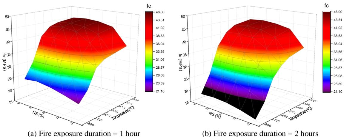
Fig.2 Compressive strengths (Cement Replacement with NS)
