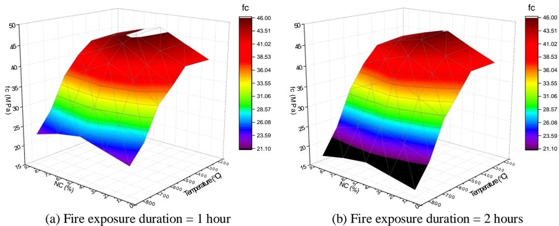
Fig.3 Compressive strengths (Cement Replacement with NC)
