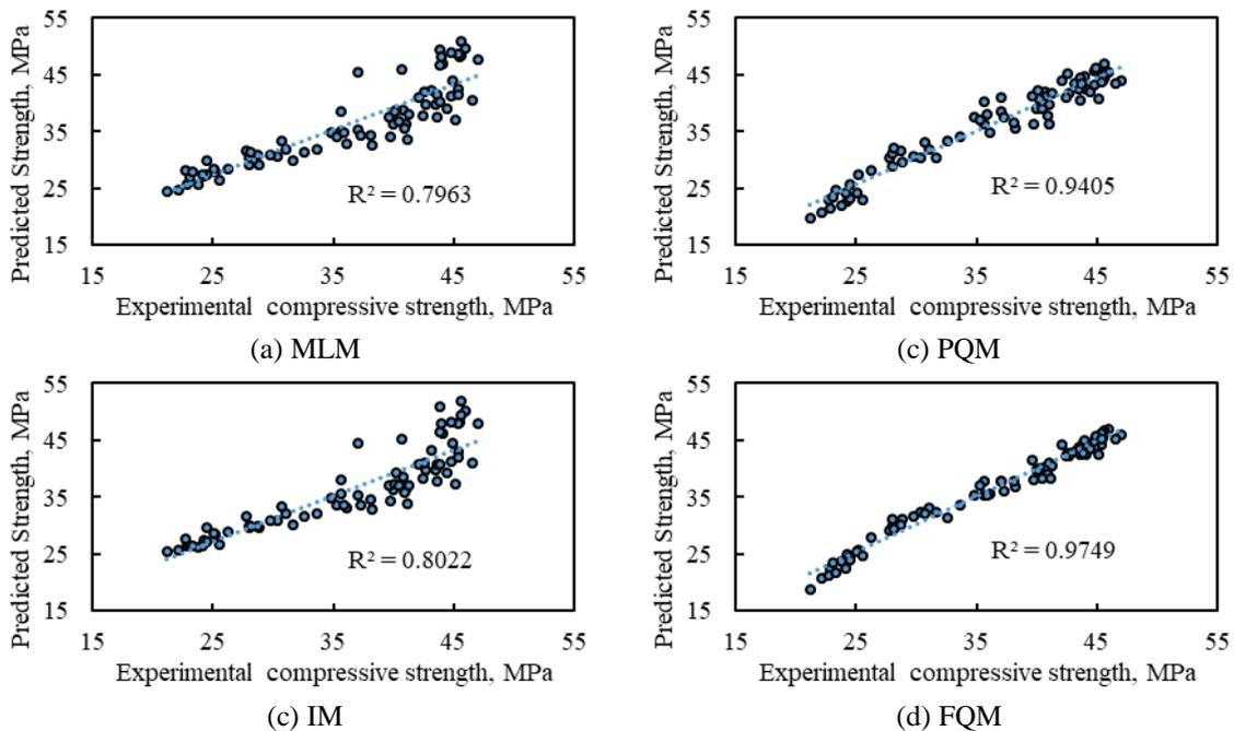
**Fig.8** Experimental values versus predicted values (1-hour of fire exposure)
