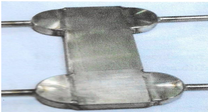
Figure 2 – Final shape of a microchannel heat exchanger (PCHE) (Reference [3]).
