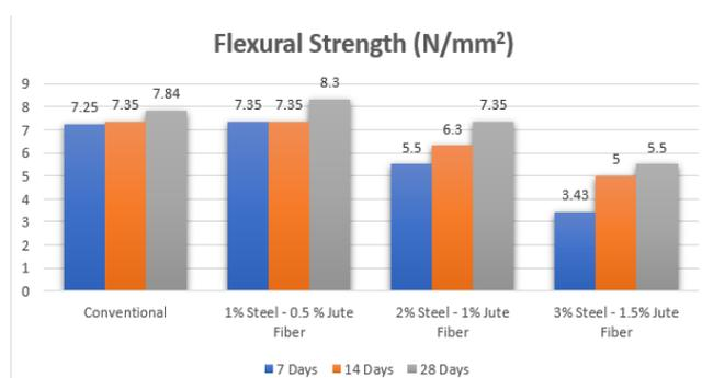
**Figure no 6: Flexural Strength Comparison Chart**
