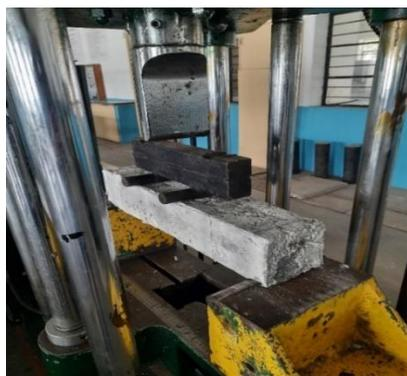
Figure no 3: Flexural Strength Test
