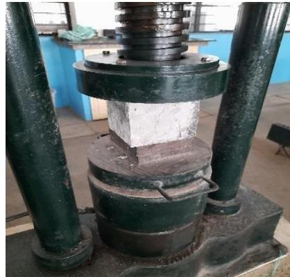
**Figure no 1:** Compressive Strength Test
