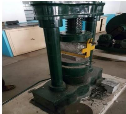
**Figure no 2:** Split Tensile Strength Test
