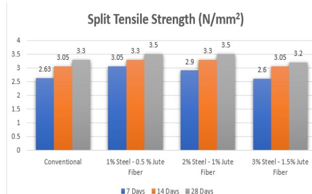
**Figure no 5:** Split Tensile Strength Test Comparison Chart
