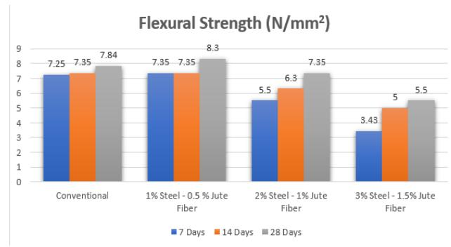
**Figure no 6:** Flexural Strength Comparison Chart
