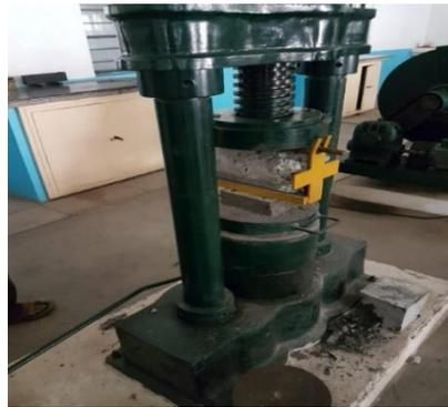
**Figure no 2:** Split Tensile Strength Test
