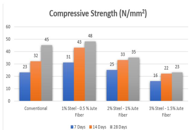
Figure no 4: Compressive Strength Test Comparison Chart
