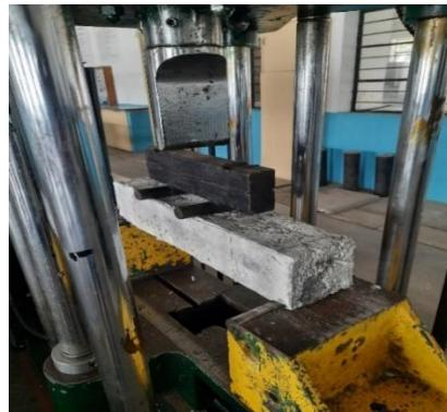
**Figure no 3:** Flexural Strength Test
