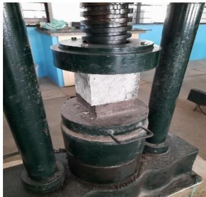
**Figure no 1:** Compressive Strength Test
