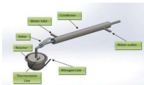
Figure 2: Opaque reactor with condenser
