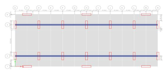
Figure (9): Plan of Girder System to Transfer Floor.
