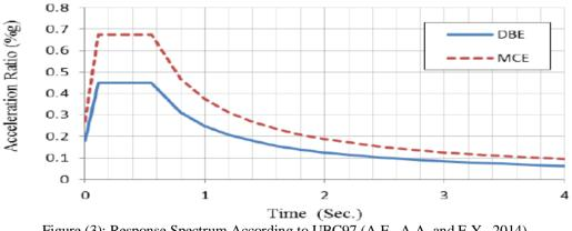
Figure (3): Response Spectrum According to UBC97 (A.E., A.A. and E.Y., 2014).
