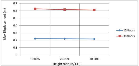
Figure 19: Comparison between the Maximum Displacement Values of 15 and 30 Floors Buildings with Transfer System.
