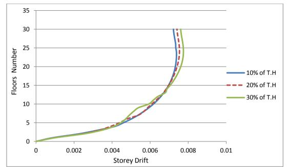
Figure (17): Storey-Drift in Y Direction for a Building 30 Floors with Transfer Floor (Girder System) at 10, 20, and 30 % of the Total Height of the Building, respectively.
