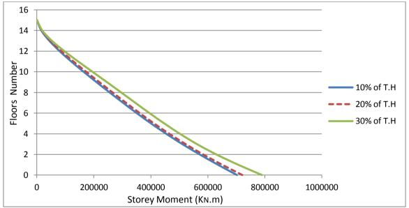
Figure (14): Storey-Moment in Y Direction for a Building 15 Floors with Transfer Floor (Girder System) at 10, 20, and 30 % of the Total Height of the Building, respectively.
