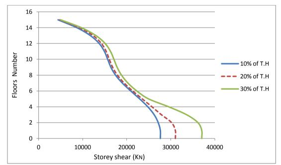
Figure (12): Storey-Shear in Y Direction for a Building 15 Floors with Transfer Floor (Girder System) at 10, 20, and 30 % of the Total Height of the Building, respectively.
