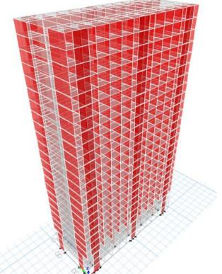
Figure (2): The Prototype Model with Transfer Floor at 10% of Building Height.
