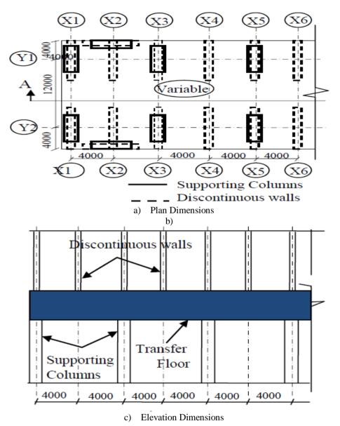
Figure (1): Finite Element Model with Transfer Floor: a) Plan Dimensions and
