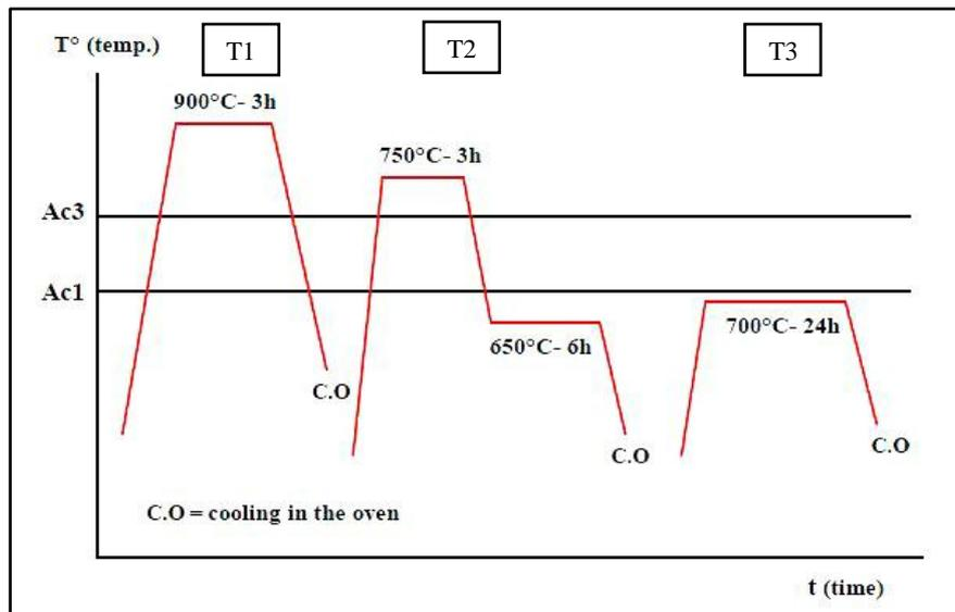
**Figure 1.** Spheroidizing heat treatment program carried out on the two types of steels used in the research
