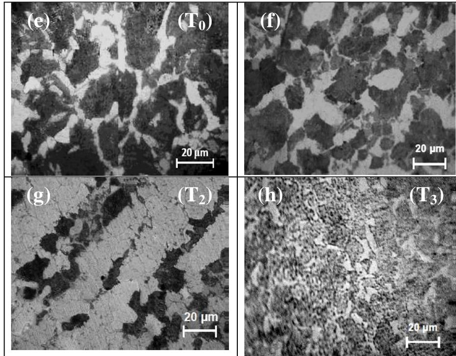
**Figure 9.** Microstructures at optical level of samples the two types of steels, subjected to different spheroidized conditions; (a), (b), (c), (d): SAE 1040; (e), (f), (g), (h): SAE 1050.
