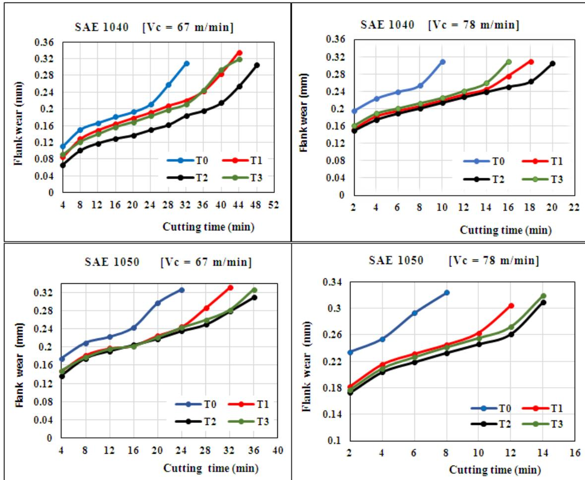
Figure 4. Wear measurement graphs on the flank wear of the HSS cutting tool, when turning SAE 1040 and SAE 1050 steel bars, under spheroidized treatments using cutting speeds: 67m/min, and 78 m/min.
