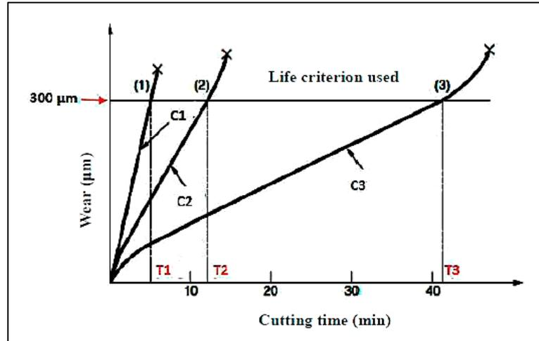
**Figure 2.** Illustrative graph, that explains, how the tool life has been obtained. Each curve represents a wear curve in machining under a preset condition.
