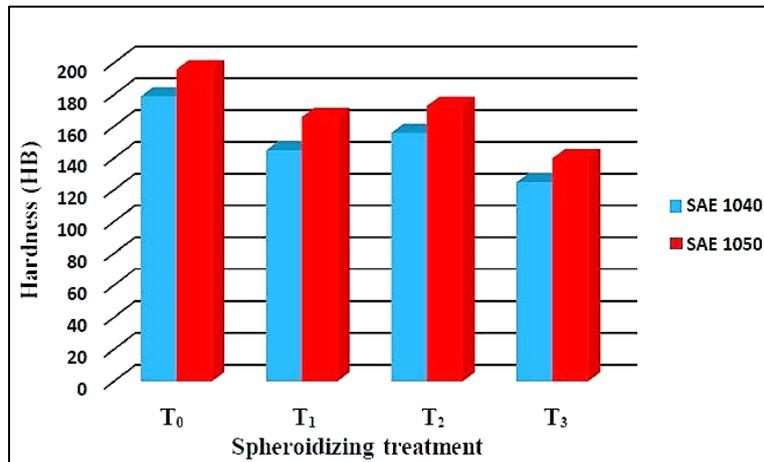
**Figure 3.** Comparative graph showing the variation in hardness of the two types of steel: SAE 1040 and SAE 1050 subjected to different types of spheroidized heat treatments.
