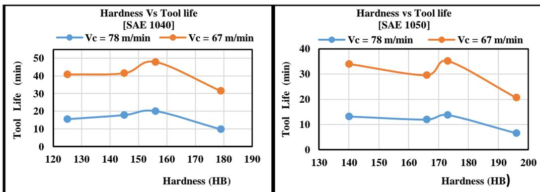
Figure 8. Tool life trend curves as a function of the hardness of the steels: SAE1040 / 1050, and cutting speeds used in machining
