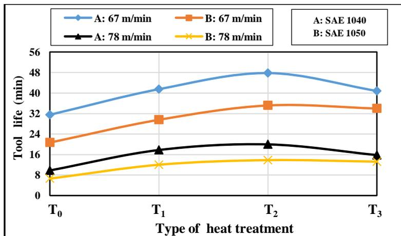
Figure 6. Graphs that indicate variation of tool life with respect the types of spheroidized heat treatment.
