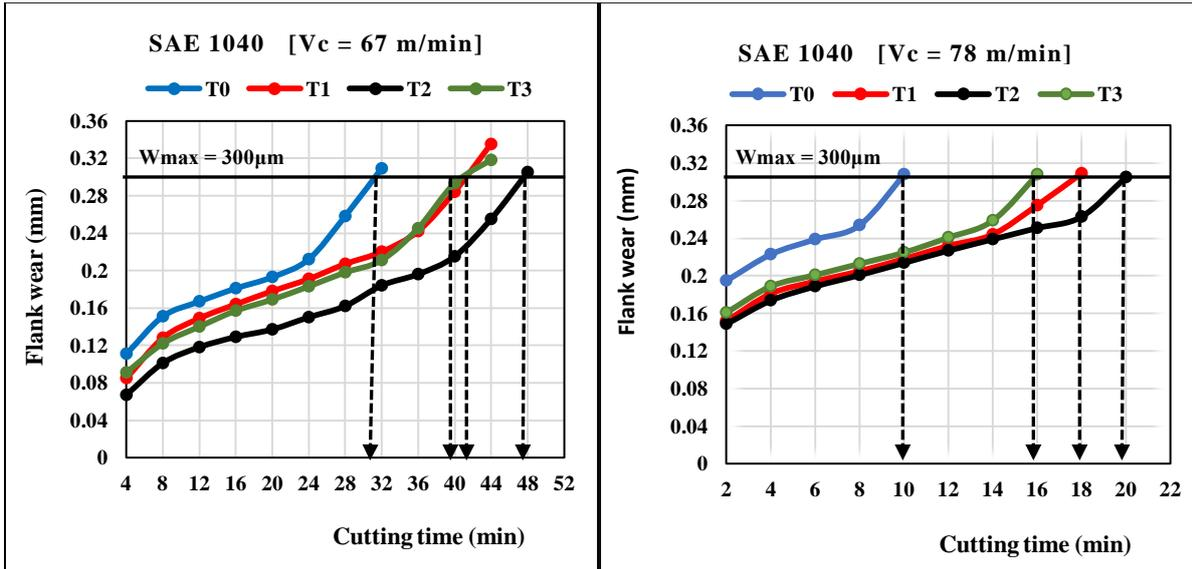
Figure 5. Graphs that indicate the procedure followed to determine tool life of the HSS cutting tool, for turning spheroidized SAE 1040 steel using cutting speeds: 67 and 78 m / min. (S=Vc)
