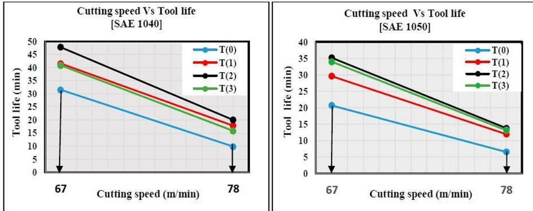
Figure 7. Tool life trend curves as a function of cutting speed for turning SAE 1040 and SAE 1050 steel bars.
