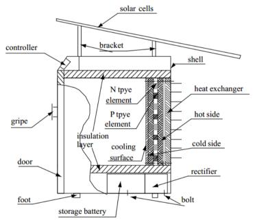
Figure No. 6: Schematic of Solar Cells driven Thermoelectric Refrigerator
