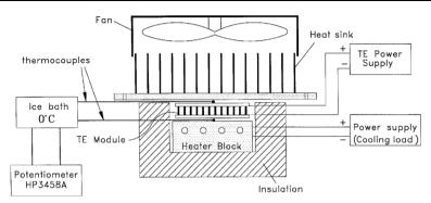
Figure No. 3: Schematic of Thermoelectric Cooler
