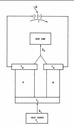
Figure No. 2: A Thermoelectric Refrigerator
