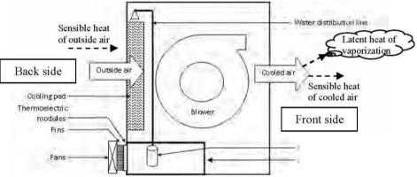
Figure No. 4: The Combined TE-Direct Evaporative Air Cooler
