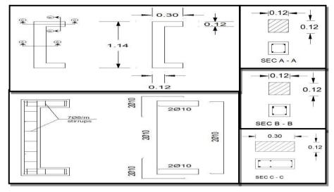
Fig. (6): Concrete Dimensions And Reinforcement Details For Columns (C1, C2, C3, C4, C9, C10, C11andC12)
