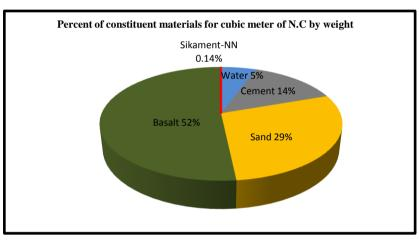
Fig. (5): Percent of Constituent Materials for Cubic Meter of N.C by Weight
