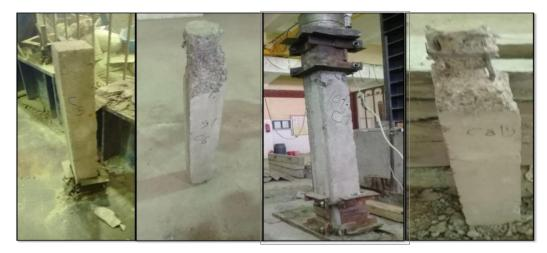
Fig. (19): Mode Failure Of The Tested Columns Of Group C
