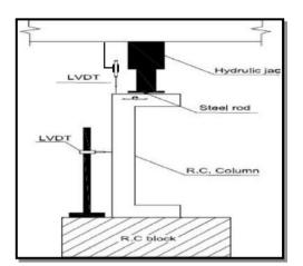
**Fig. (11):** Position of Group (B& C) Columns under Loading Jack
