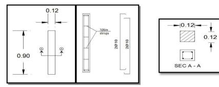
Fig.(7): Concrete DimensionsAnd Reinforcement Details For Columns (C5, C6, C7 and C8)
