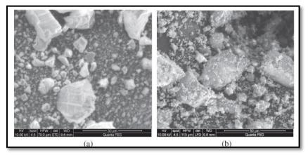
Fig. (1): SEM image appears powder morphology, (a) white and (b) brown eggshells
