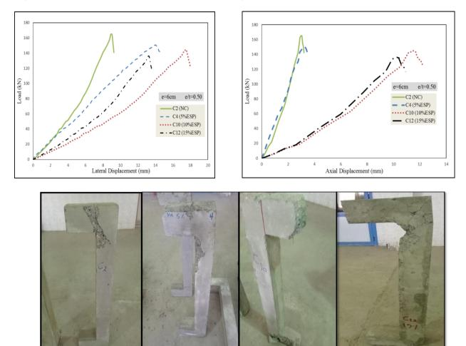
Fig. (17): Relation between Load and Lateral Deflection Fig. (18): Relation between Load and Axial Deflection
