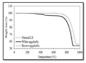
Fig. (2):TGA analysis for limestone, white and brown powders [4]
