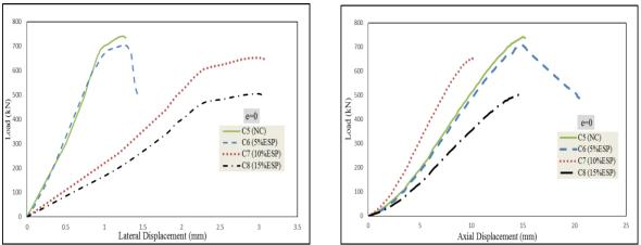
Fig. (20): Relation between Load and Lateral Deflection Fig. (21): Relation between Load and Axial Deflection
