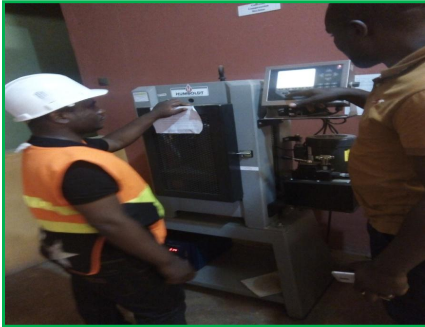
Fig. 10: Researcher with assistant crushing test specimens at Digital compression test machine at Bambuiy Geotechnical Laboratory
