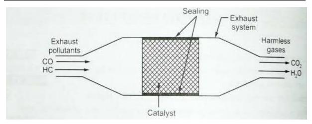
2. Three-way Catalytic converter: Three-way catalytic converter treats Carbon monoxide and unburnt hydrocarbon similarly as Two-way catalytic converter. Additionally, Here reduction of nitrogen oxides to nitrogen and oxygen also take place:
