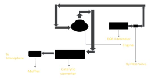
The exhaust gas enters into the catalytic converter where it firstly reacts with a reduction honeycomb substrate which is coated by platinum and rhodium catalyst. Here harmful NOx emission in converted into nitrogen and oxygen which are not harmful to nature. Now these exhaust gases further reacts with oxidation honeycomb substrate which is coated with platinum and palladium catalysts. Here harmful HC and CO are concerted in less harmful water vapor and carbon dioxide.
