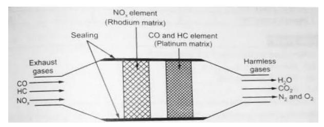
**3. Dual bed Catalytic converter:** A dual bed catalytic converter is combination of a two-way and a three-way catalytic converter combined in a single housing with a air chamber between them. The exhaust gases are firstly reduced to remove NOx emission from the exhaust gases and then these exhaust gases passes through the air chamber present between them. Here, sufficient amount of air is added for the oxidation of HC and CO present in exhaust gases.
