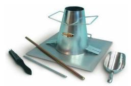
Figure-2 Slump Test Apparatus
