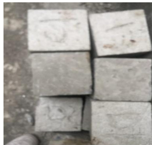
Fig. 4 Compression failure samples
