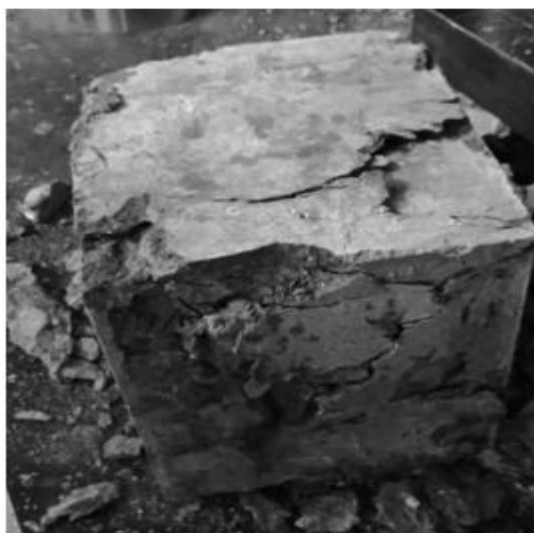
Fig. 4 Compression failure samples
