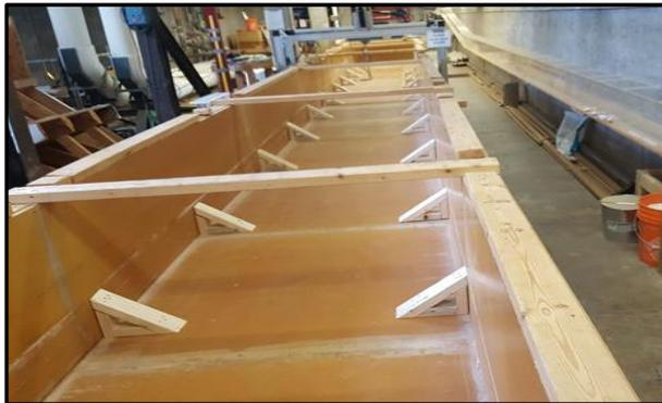
**Photo no 2:** Timber flume during construction
