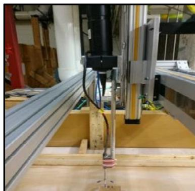
**Photo no 5:** Down-Looking ADV in Down-Looking orientation
