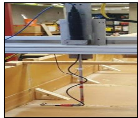
**Photo no 6:** Side-Looking ADV in Up-Looking orientation
