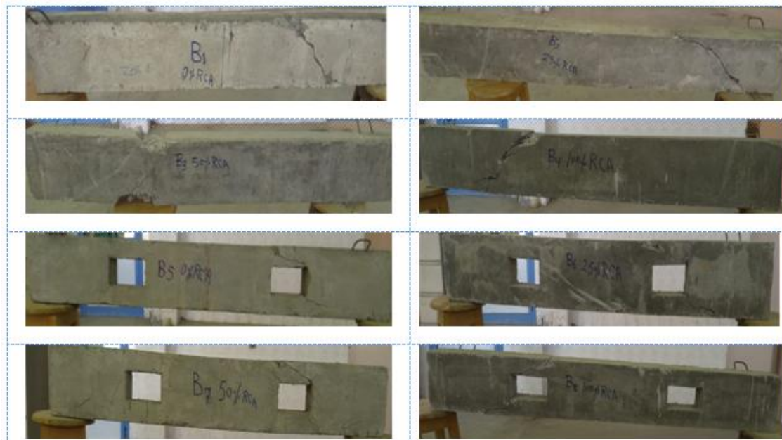
Fig. 5 Crack pattern for the tested beams
