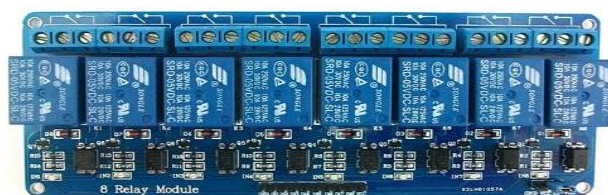
Fig. 11 Relay interface board
