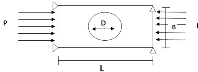
Fig. 1- A rectangular plate with a circular opening subjected to a compressive force
