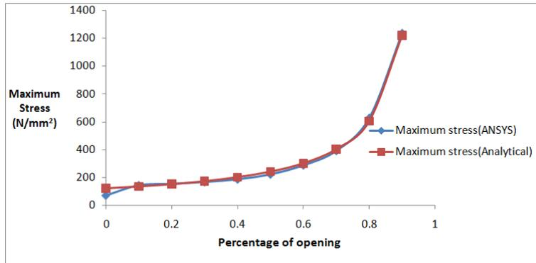
Fig. 4- Comparison of analytical and numerical values of maximum stress for different ratio of openings
