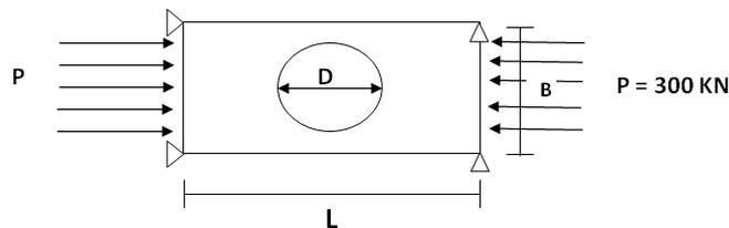
Fig. 3- A plate of finite width for numerical study
