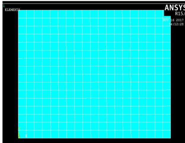
Fig. 6- A Meshed rectangular plate ready for analysis with ANSYS
