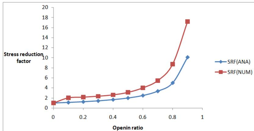
Fig. 5- Comparison of analytical and numerical values of stress reduction factors for different ratio of openings
