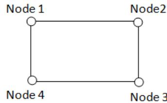
Fig. 2- A four node finite element used in this study
