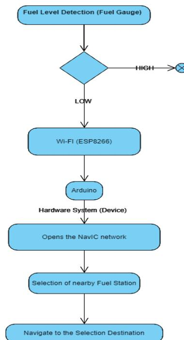
**Fig.1** flowchart of fuel detection and navigation
