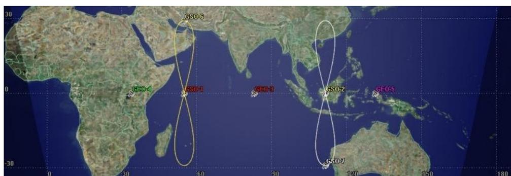
**Fig .2** positioning of IRNSS
