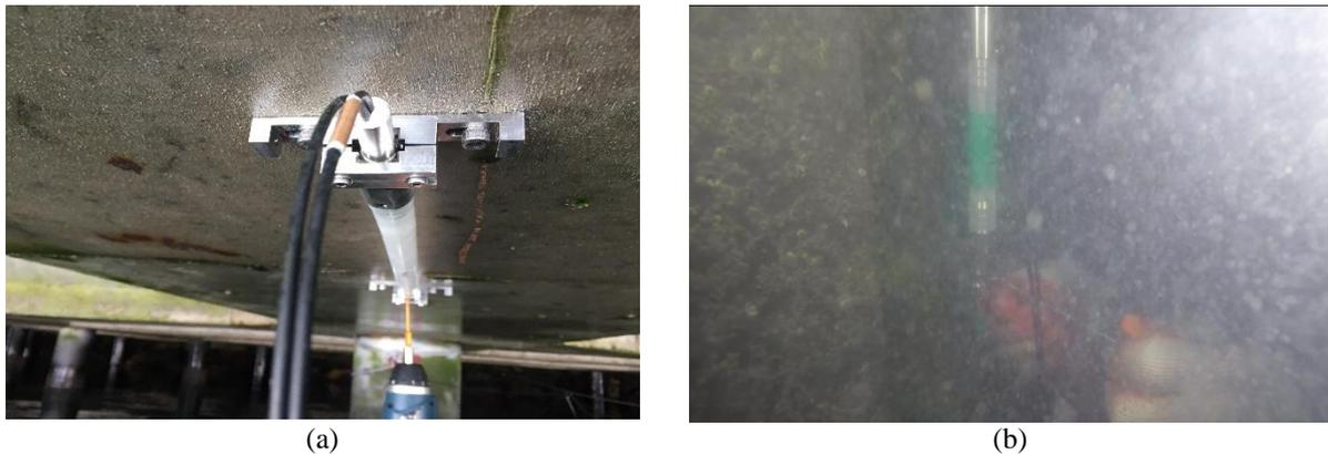
**Figure no 4:**The FBG Sensors Installed (a) under the harbor structure and (b) underwater
