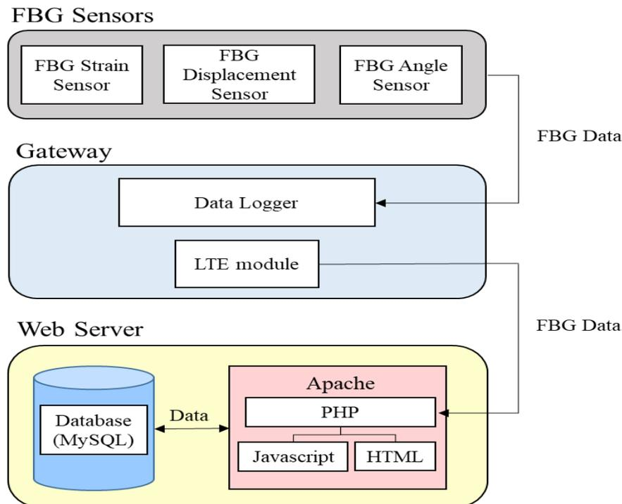
**Figure no 3:**System Diagram of the IoT based Gravity Type Harbor Structure Health Monitoring Platform
