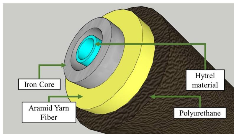
**Figure no 1:** Designed Cable for FBG sensors
