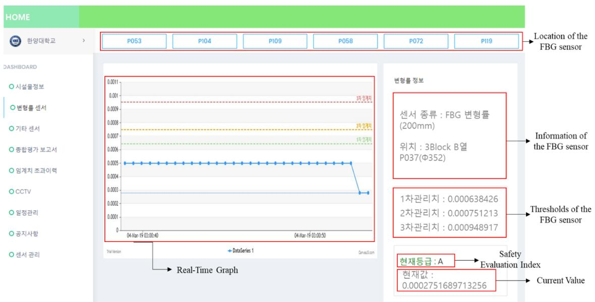
Figure no 6: Detailed Monitoring Page of the Web Server for IoT based Gravity Type Harbor Structure Health Monitoring Platform
