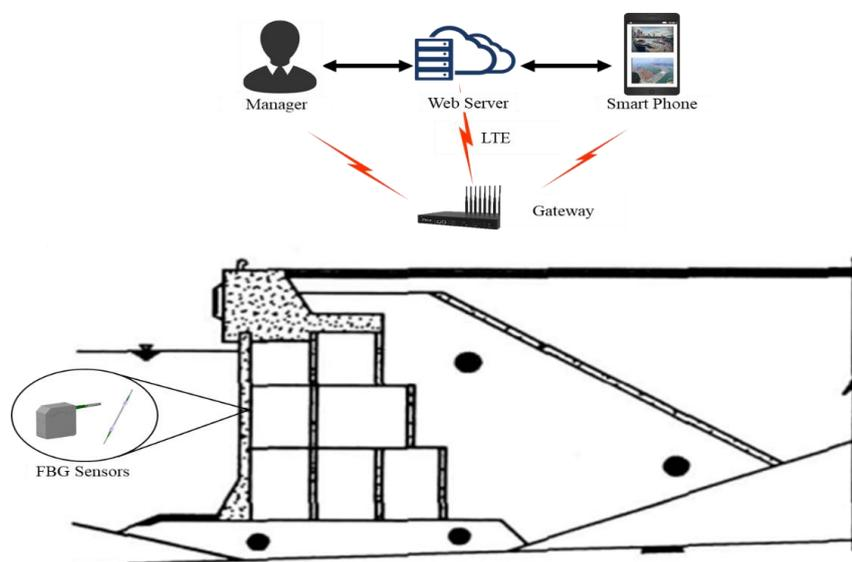
**Figure no 2:**Configuration Diagram of the IoT based Gravity Type Harbor Structure Health Monitoring Platform
