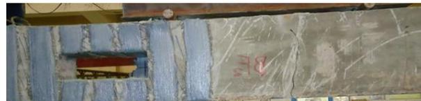
**(e) Crack pattern of the beam (BF2).**
