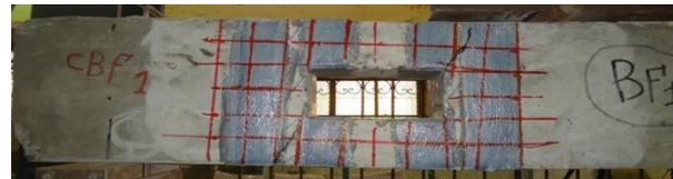
**(c) Crack pattern of the beam (BF1).**
