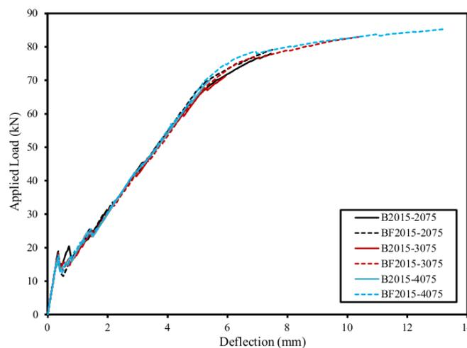
**Figure (10):** Load-Deflection relation of the beams in the second group.
