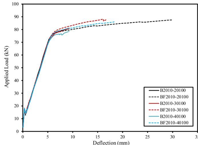
**Figure (9):** Load-Deflection relation of the beams in the first group.
