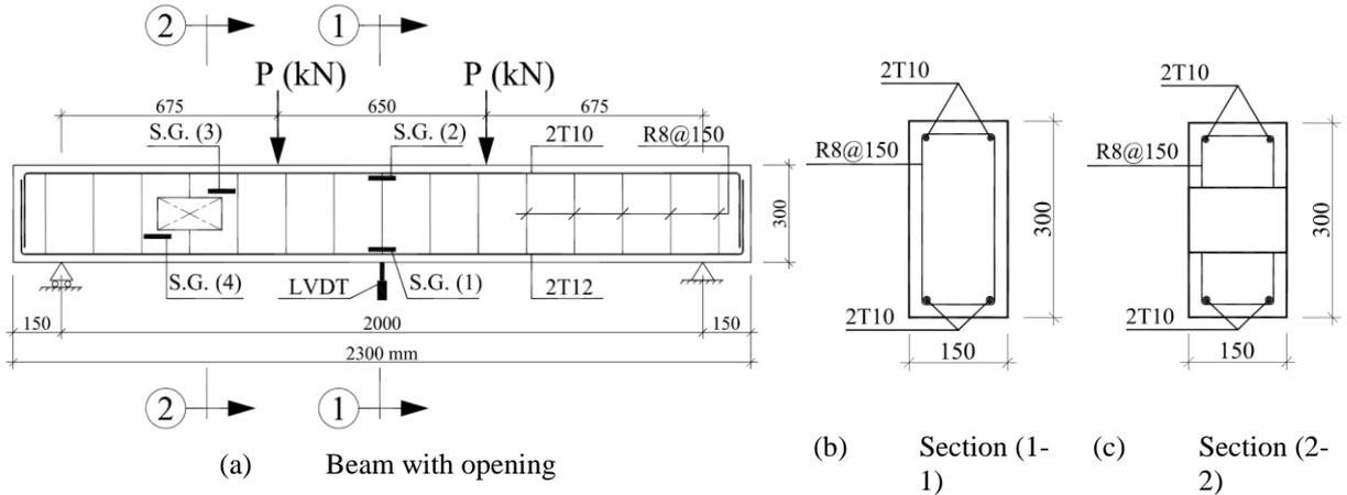
Figure (2): Geometric configuration, reinforcement details and, loading scheme of the beams with openings.
