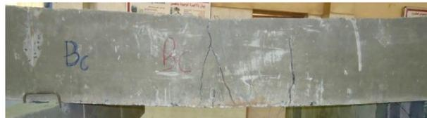
**(a) Crack pattern of the control beam (CB).**
