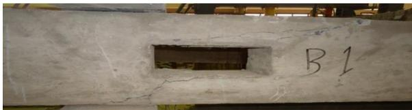
**(b) Crack pattern of the beam (B1).**
