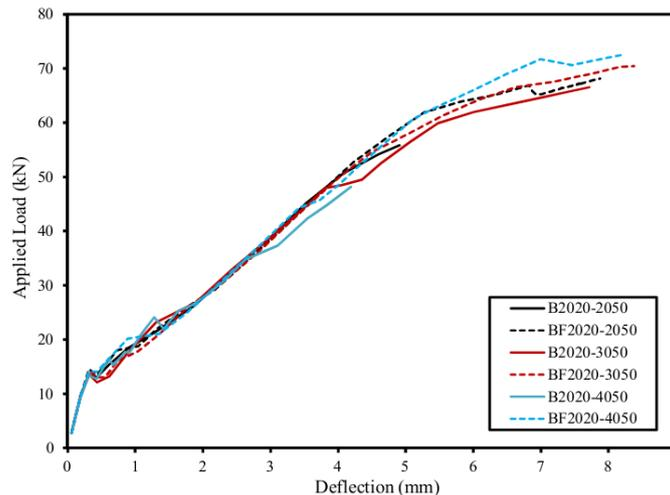
**Figure (11):** Load-Deflection relation of the beams in the third group.
