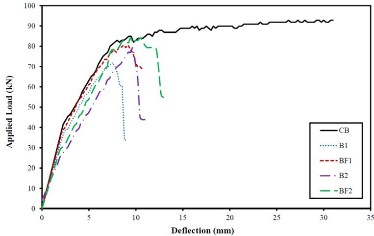
Figure (5): Comparison between the Load-Deflection relations of the experimentally tested beams.
