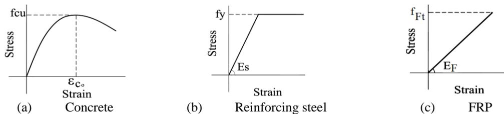
**Figure (6):** Schematic representation for the constitutive material models for (a) concrete, (b) reinforcing steel and, (c) FRP.
