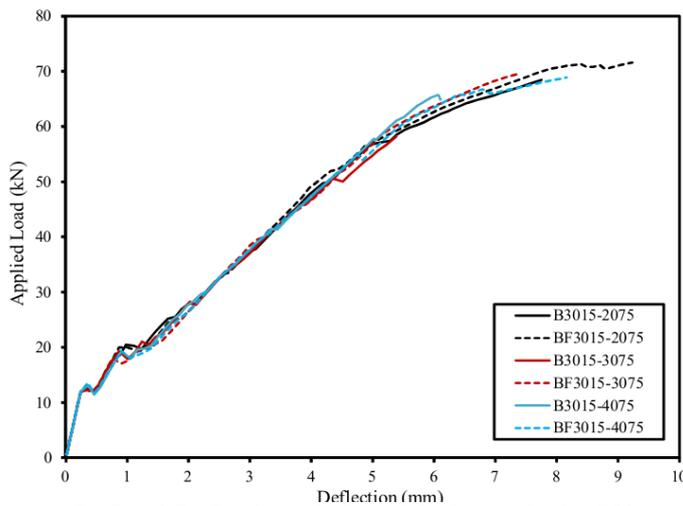
Figure (13): Load-Deflection relation of the beams in the fifth group.
