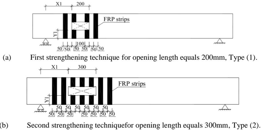
Figure (8): The two FRP strengthening techniques: (a) Type (1) and, (b) Type (2).
