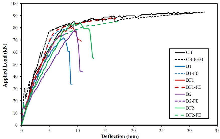
**Figure (7):** Comparison between the Load-Deflection relations of the FE models and the tested beams.
