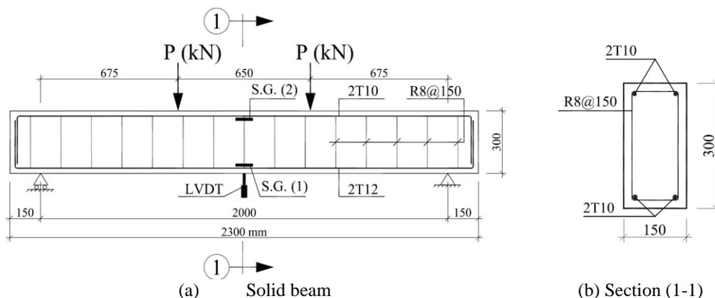
**Figure (1):** Geometric configuration, reinforcement details and, loading scheme of the Control Beam, CB.
