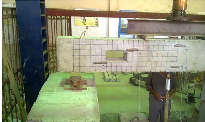
**Figure (3):** The loading frame and setting out of the tested beams.
