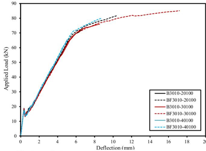
Figure (12): Load-Deflection relation of the beams in the fourth group.
