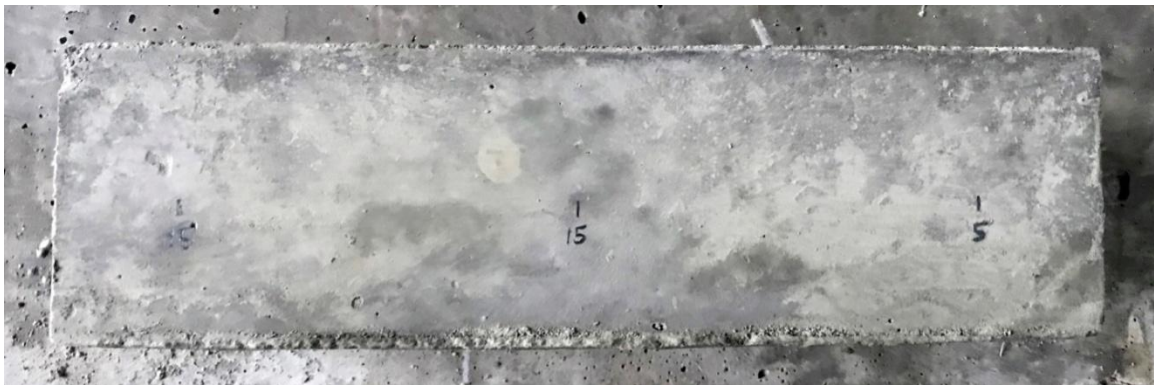
Figure 2: Drilling locations for cement concrete sample powder.
