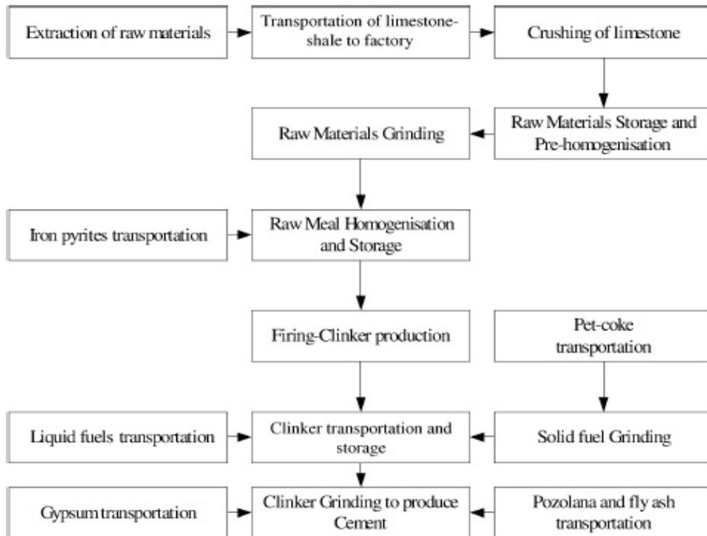
Figure 1. Cement production stages
