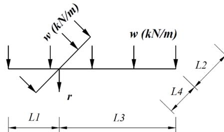
Figure 3: Plate structural model
