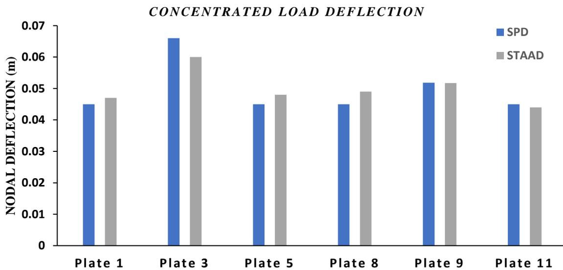
Figure 25: Nodal deflection results for concentrated loading case
