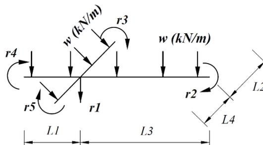
Figure 6: Structural model for simply supported boundaries
