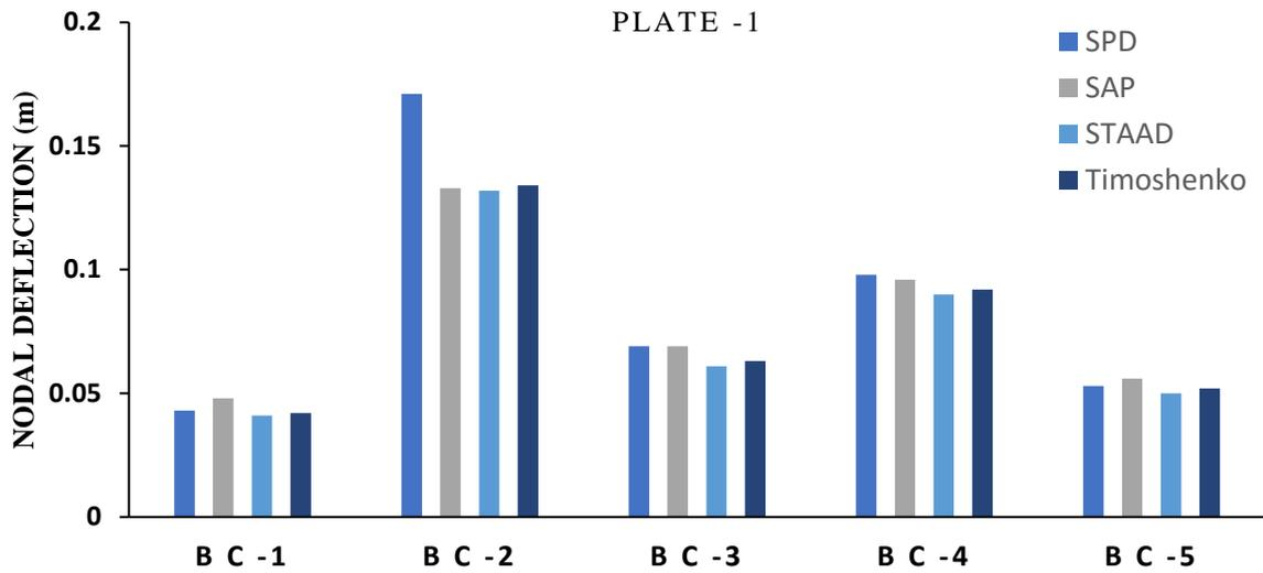
Figure 22: Nodal displacement comparison of Plate -1 loaded uniformly
