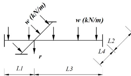
Figure 4: Plate structural model for fixed boundaries
