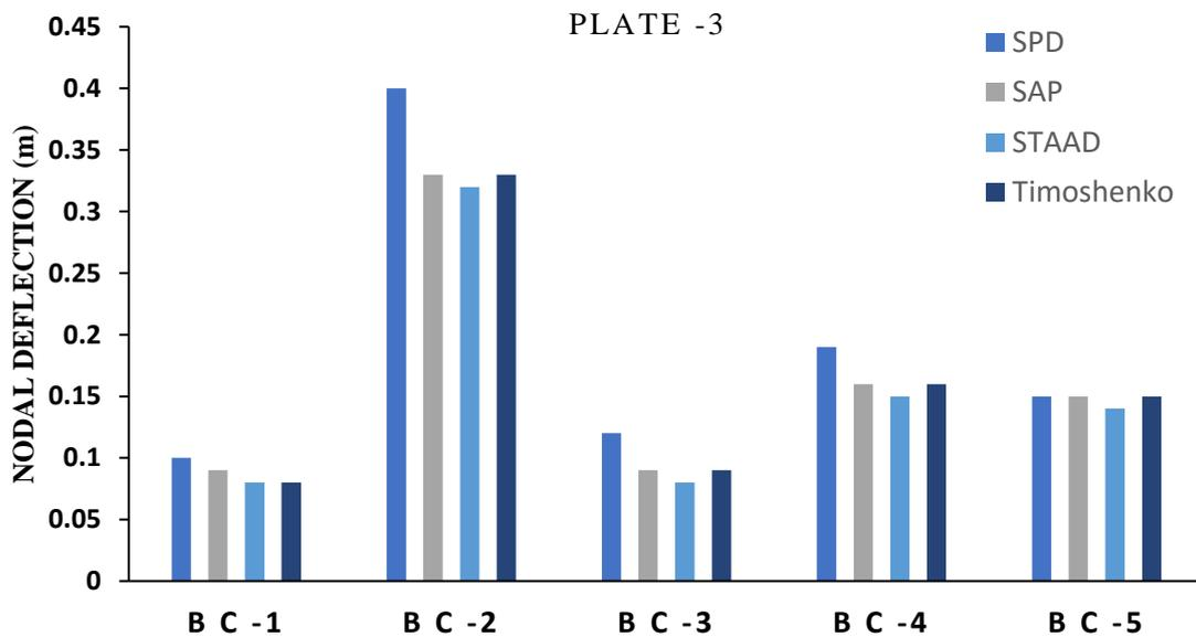
Figure 23: Nodal displacement comparison of Plate -3 loaded uniformly
