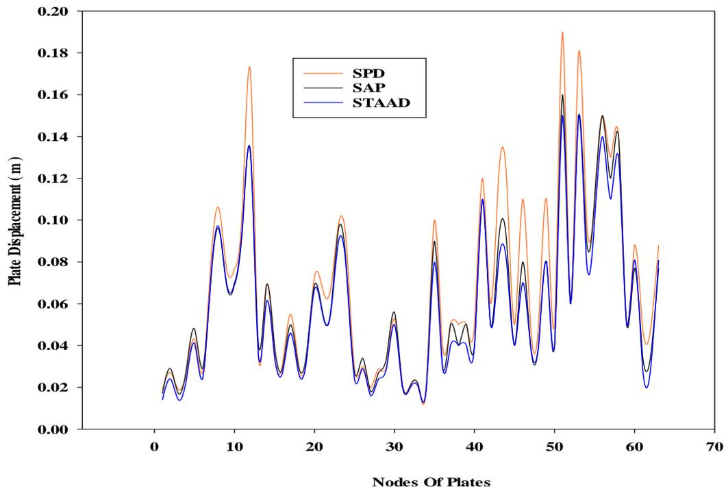
Figure 21: Nodal Displacements Comparison of Plates Loaded uniformly
