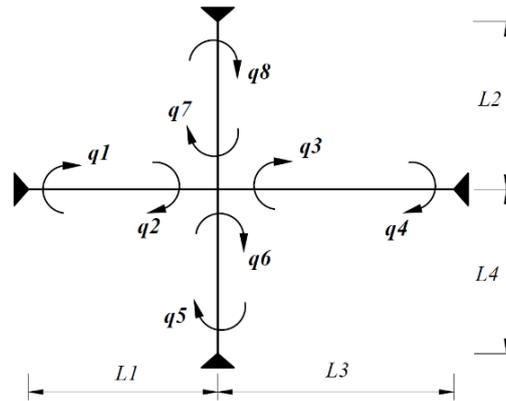
Figure 7: Plate internal element forces for simply-supported boundaries
