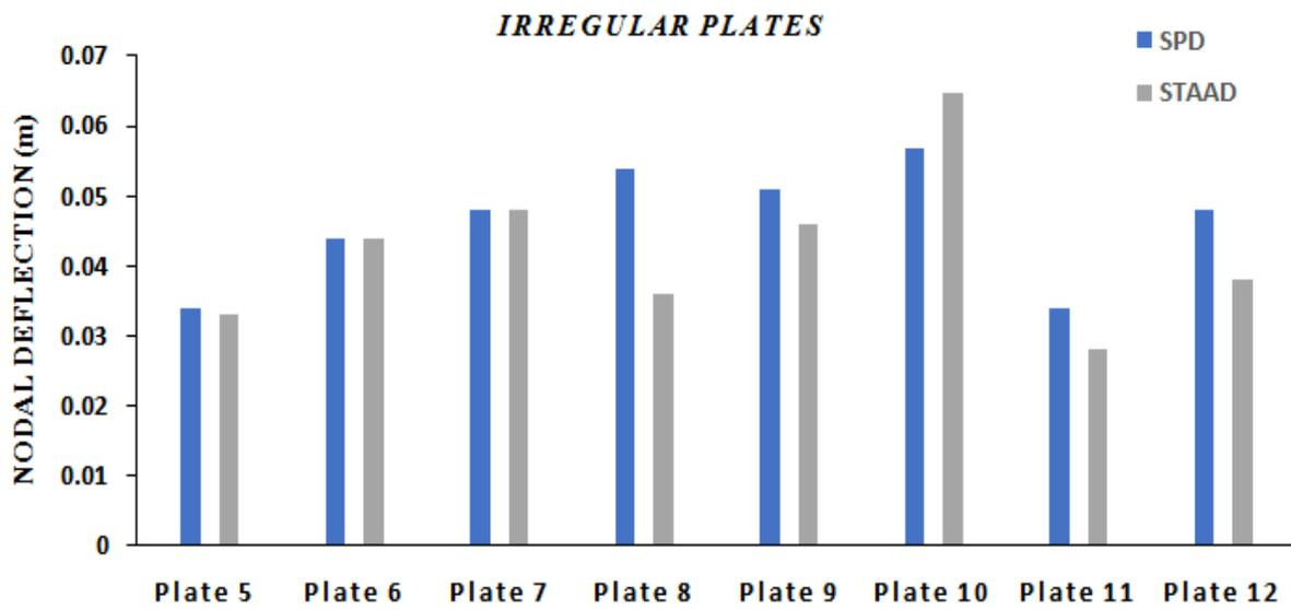
Figure 24: Nodal displacement comparison for Irregular plates loaded uniformly
