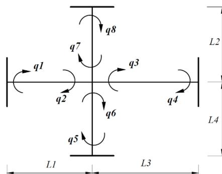
Figure 5: Plate internal element forces for fixed boundaries
