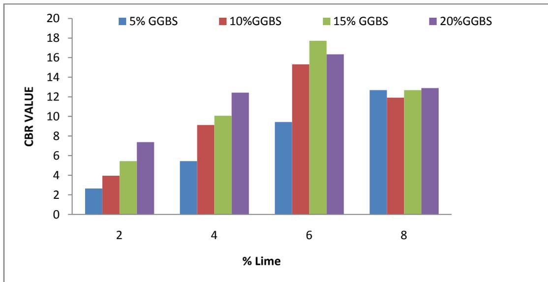
Fig 13 Bar chart showing CBR variation for different combinations of Lime with (5%, 10%, 15% and 20%) GGBS
