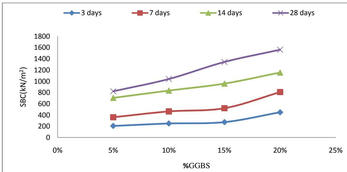
Fig 25 Graph showing SBC vs %GGBS for 8% Lime
