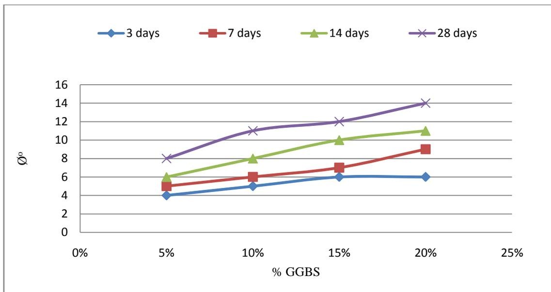
Fig 17 showing variation of 'phi' with variation of GGBS for different curing periods for 4% Lime
