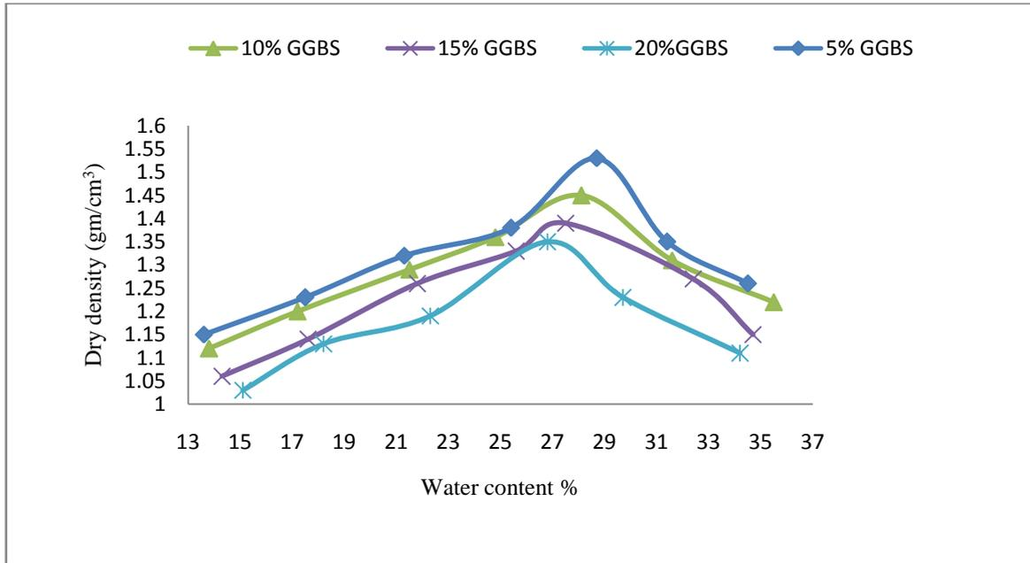
Fig 10 Graph showing compaction curves for 6% Lime with (5%, 10%, 15% and 20%) GGBS
