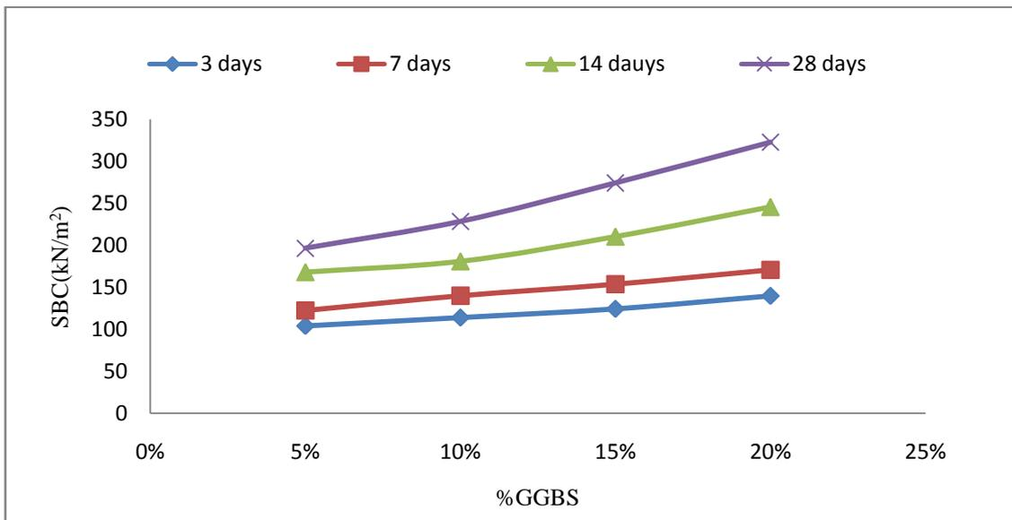
Fig 22 Graph showing SBC vs %GGBS for 2% Lime
