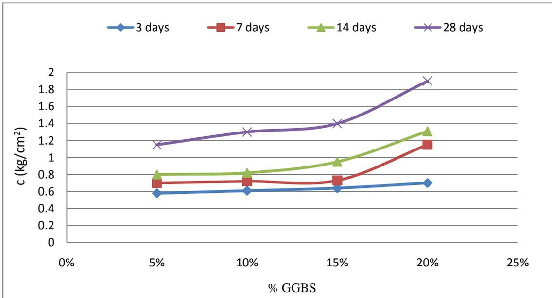
Fig 18 showing variation of 'c' with variation of GGBS for different curing periods for 6% Lime
