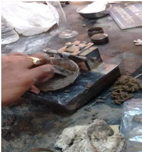
**Fig 1:** Casagrande apparatus for determination of liquid limit.
