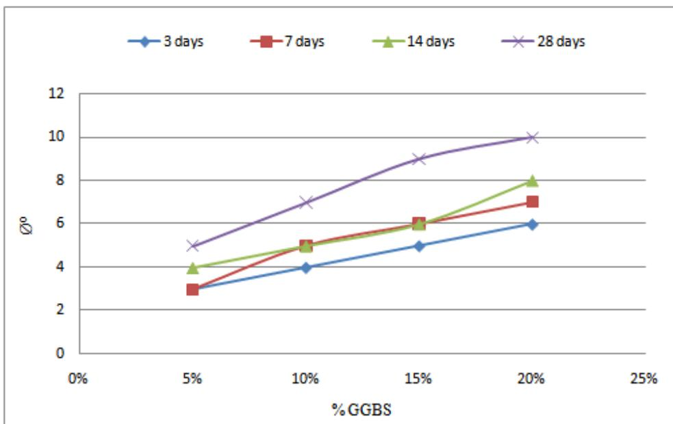
**Fig 15** showing variation of ' $\phi$ ' with variation of GGBS for different curing periods for 2% Lime
