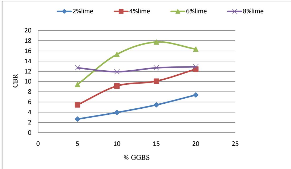
Fig 12 Graph showing CBR variation for different combinations of Lime with (5%, 10%, 15% and 20%) GGBS
