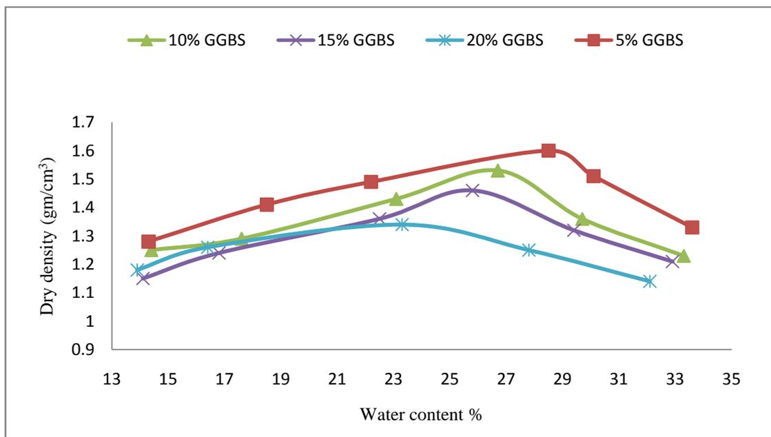
Fig 9 Graph showing compaction cures for 4% Lime with (5%, 10%, 15% and 20%) GGBS
