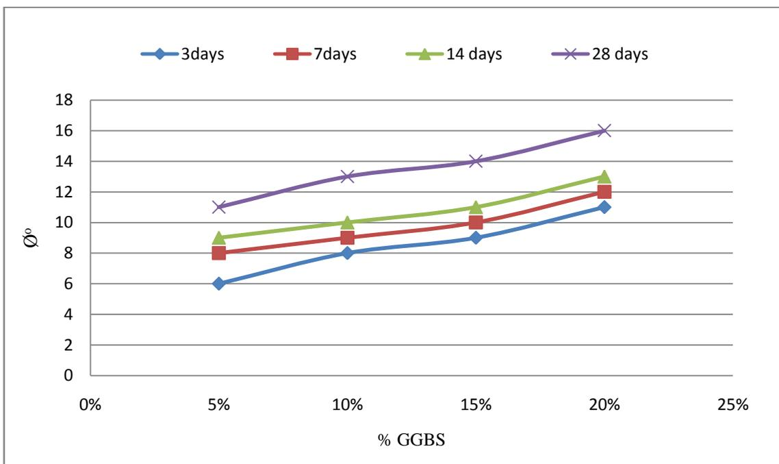
Fig 21 showing variation of ' $\phi$ ' with variation of GGBS for different curing periods for 8% Lime
