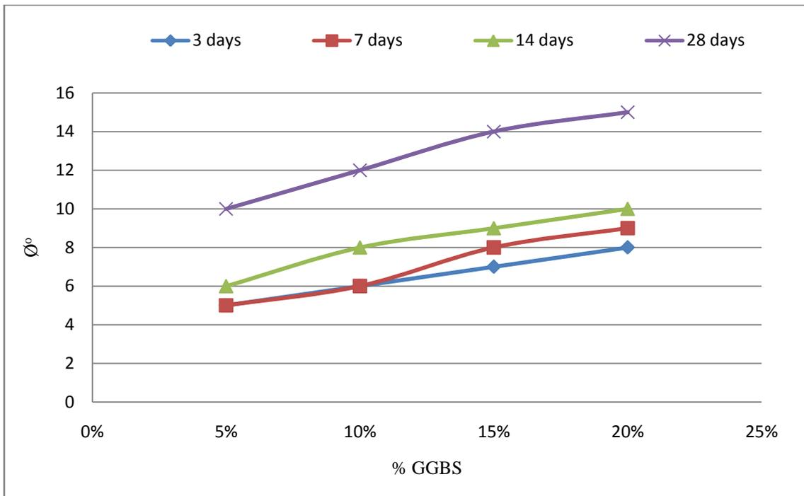
Fig 19 showing variation of '∅' with variation of GGBS for different curing periods for 6% Lime
