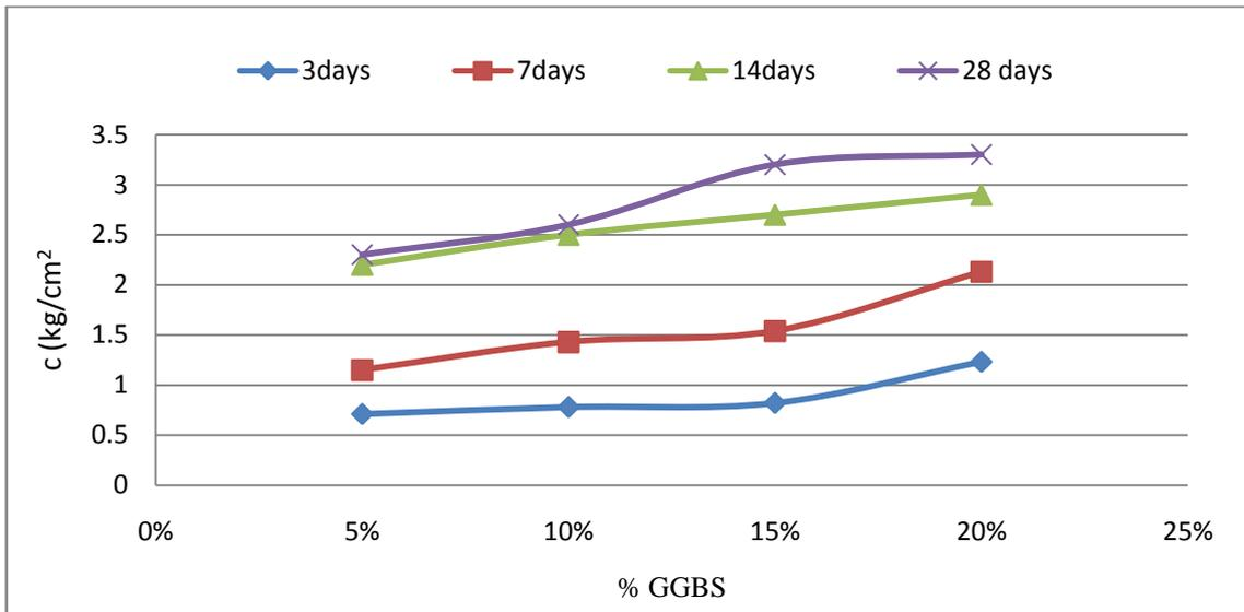
Fig 20 showing variation of 'c' with variation of GGBS for different curing periods for 8% Lime
