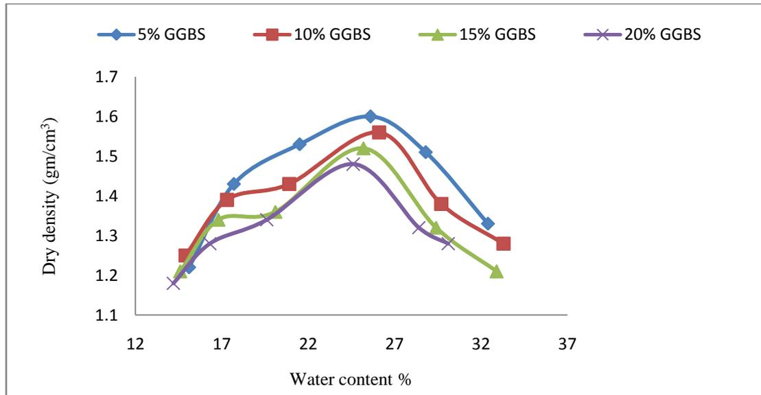
Fig 8 Graph showing compaction cures for 2% Lime with (5%, 10%, 15% and 20%) GGBS
