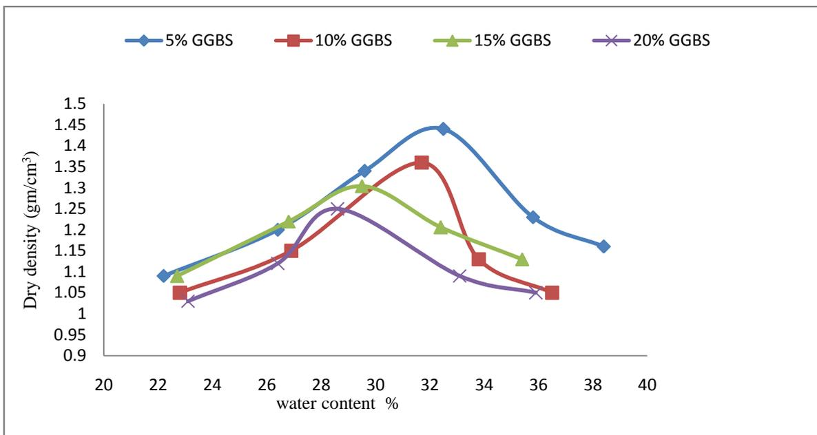
Fig 11 Graph showing compaction curves for 8% Lime with (5%, 10%, 15% and 20%) GGBS
