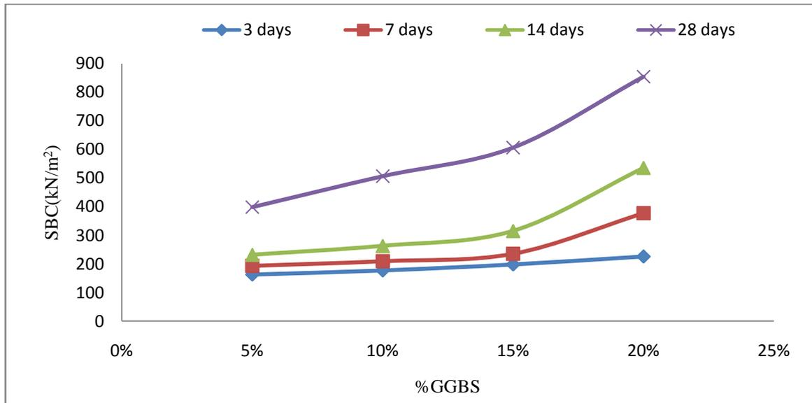
Fig 24 Graph showing SBC vs %GGBS for 6% Lime
