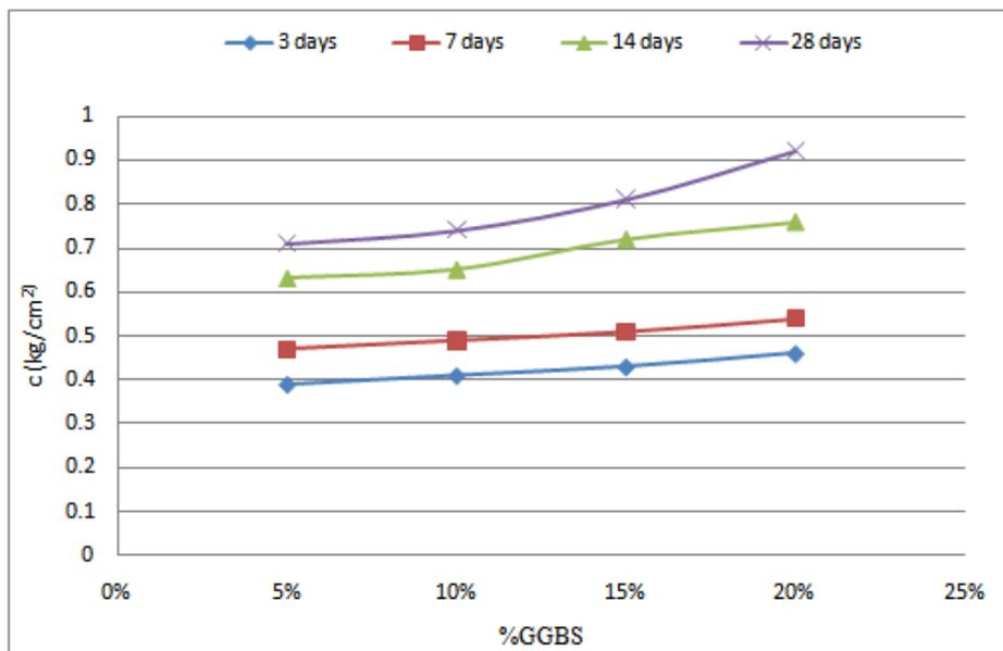
**Fig 14** showing variation of ' $c$ ' with variation of GGBS for different curing periods for 2% Lime
