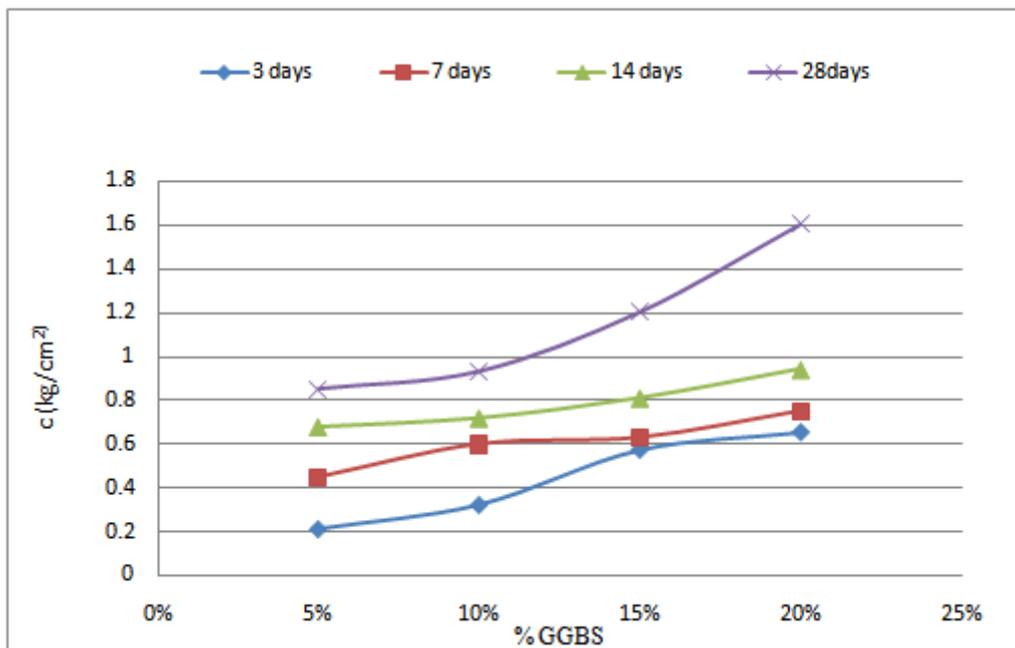
Fig 16 showing variation of 'c' with variation of GGBS for different curing periods for 4% Lime
