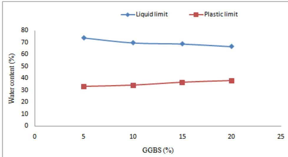
Fig 5 Variation of Liquid limit and Plastic limit for Expansive soil treated ES with 4% Lime and (5%, 10%, 15%, 20%) GGBS
