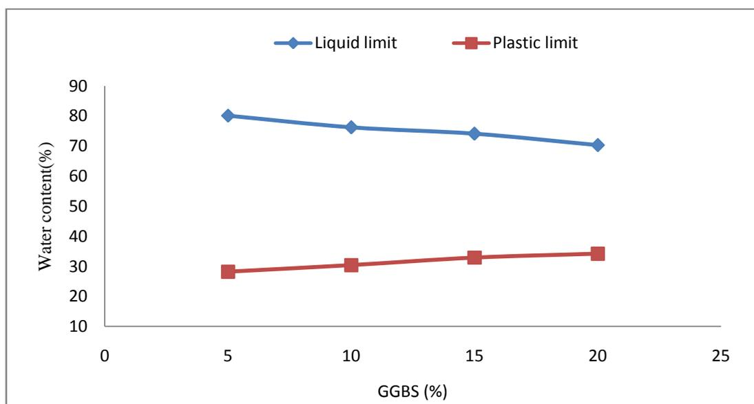
Fig 4 Variation of Liquid limit and Plastic limit for Expansive soil treated ES with 2% Lime and (5%, 10%, 15%, 20%) GGBS.
