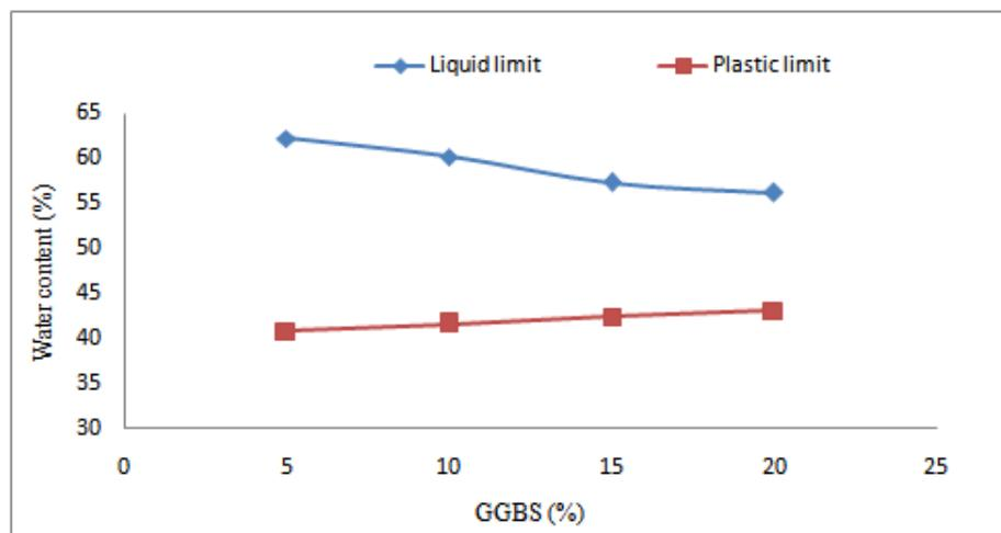
Fig 7 Variation of Liquid limit and Plastic limit for Expansive soil treated ES with 8% Lime and (5%, 10%, 15%, 20%) GGBS.
