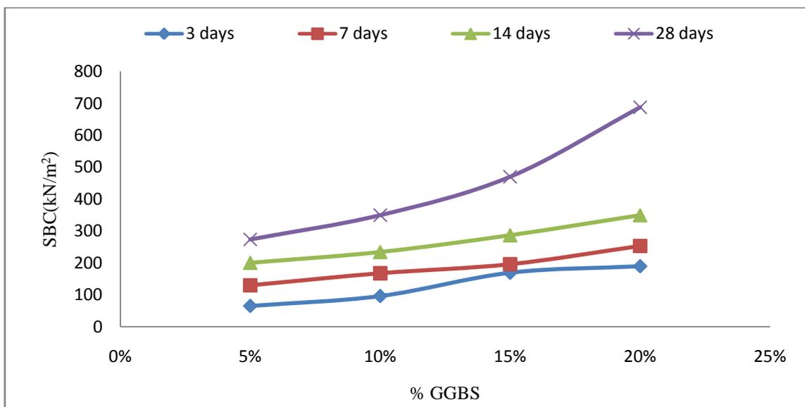
Fig 23 Graph showing SBC vs %GGBS for 4% Lime
