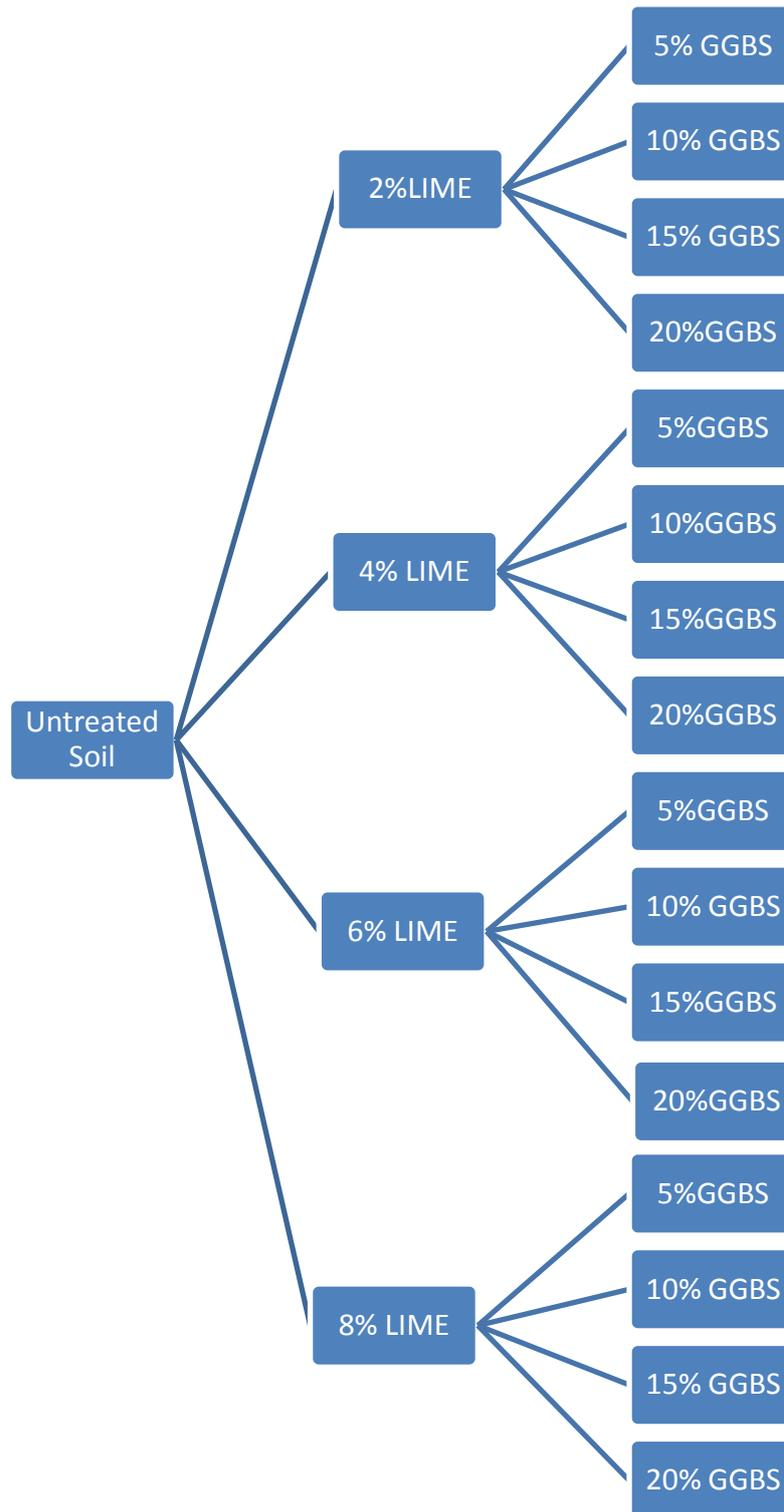
Fig 2 Flow chart showing different combinations of lime and GGBS with ES.
