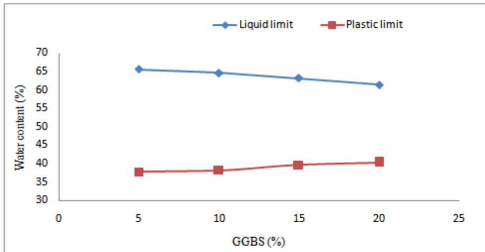
Fig 6 Variation of Liquid limit and Plastic limit for Expansive soil treated ES with 6% Lime and (5%, 10%, 15%, 20%) GGBS
