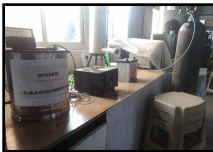
Fig No.2 Bomb Calorimeter Setup
