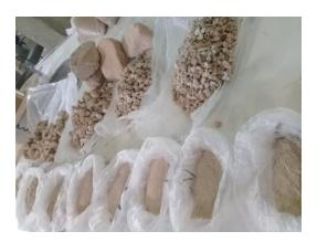
Fig (1) Recycled refractory brick after crushing and grading
