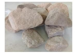
Fig (2) Recycled refractory brick
