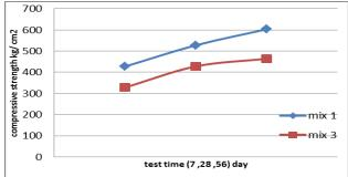
Fig (5) age of concrete with compressive strength for mix 3 (20%K,80%C)
