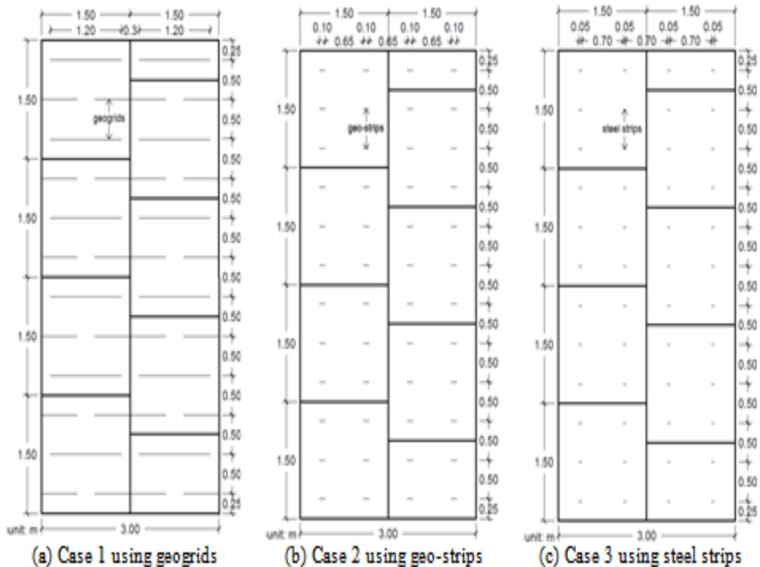
(a) Case 1 using geogrids (b) Case 2 using geo-strips (c) Case 3 using steel strips
