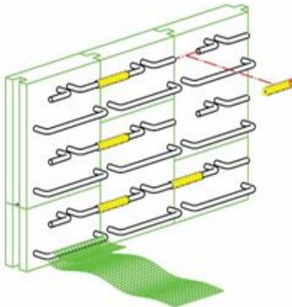
Figure 2 Modified panel type facing with steel pipe slip-on, steel bar, and geogrid connections
