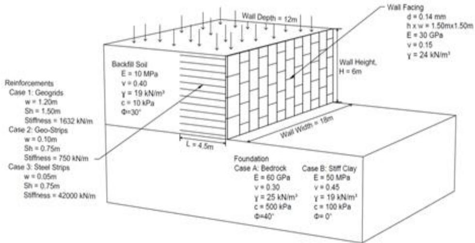
Figure 3 Numerical model of MSE wall using Plaxis 3D program
