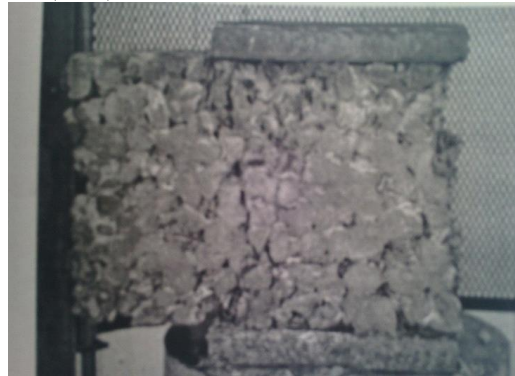
Plate 2: The failure of the no-fines concrete sample on completion of the Cube Test
