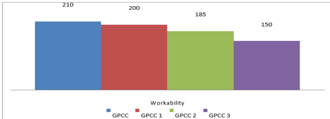
Fig -1 Comparison of Workability of GPCC without & with fibers
