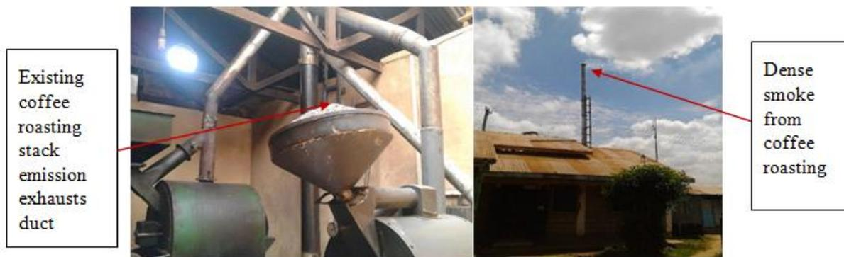
**Fig. 1.** Roaster exhaust ducts joined to one main exhaust duct extending outside the roof
