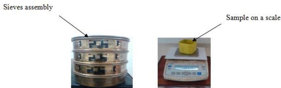
Fig.3: Sieve stack and a weigh balance at DeKUT Chemistry lab
