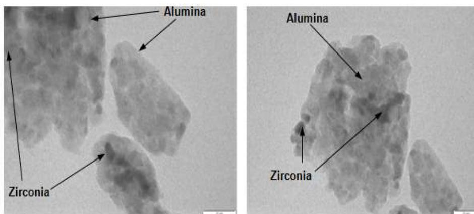
**Fig. 2.** TEM images of nanocomposite particles with 5% ZrO<sub>2</sub> in Al<sub>2</sub>O<sub>3</sub> matrix.
