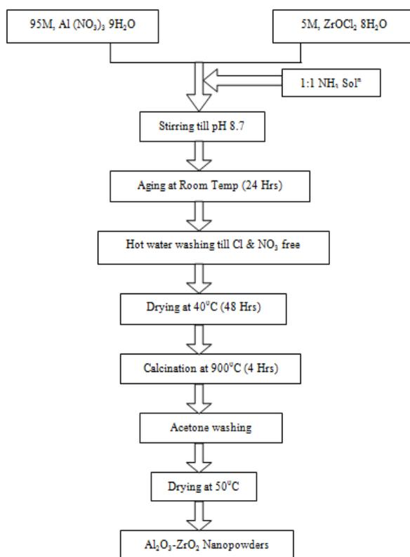
**Fig. 1.** Flowchart of sol-gel synthesis to prepare  $\text{Al}_2\text{O}_3\text{-ZrO}_2$  nanocomposite particles.
