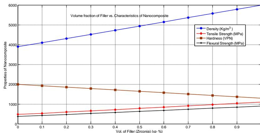
**Fig. 6.** Mechanical Properties of  $Al_2O_3$ - $ZrO_2$  nanocomposite. Density, Tensile Strength and Flexural Strength increases, whereas Hardness decreases.
