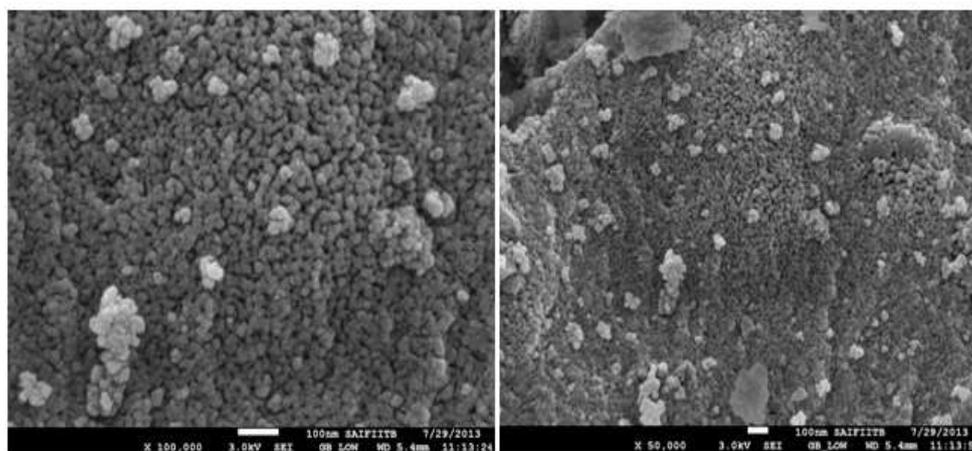
**Fig. 3.** SEM images of nanocomposite particles with 5% ZrO<sub>2</sub> in Al<sub>2</sub>O<sub>3</sub> matrix.
