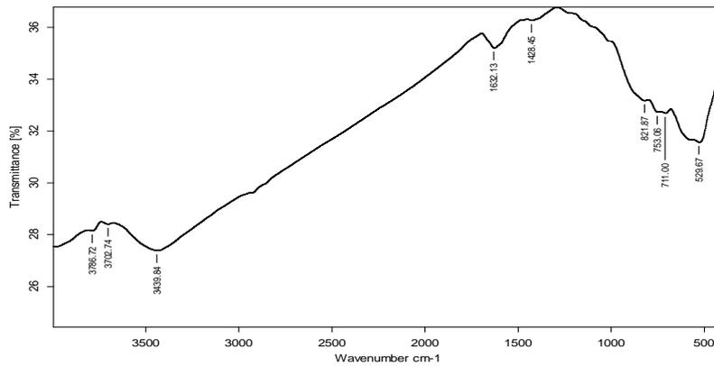
Fig. 4. FTIR spectrum of Al<sub>2</sub>O<sub>3</sub>-ZrO<sub>2</sub> nanocomposite.
