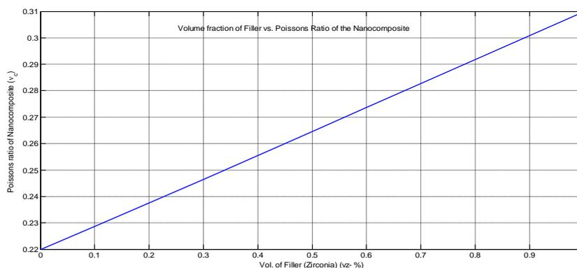
Fig. 8. Mechanical Properties of Al<sub>2</sub>O<sub>3</sub>-ZrO<sub>2</sub> nanocomposite. Poisson's Ratio directly increases with increase in volume fraction of nanofillers.
