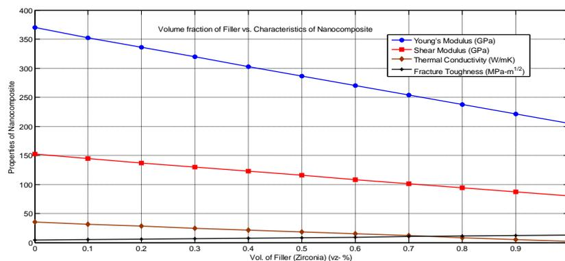
Fig. 7. Mechanical Properties of Al<sub>2</sub>O<sub>3</sub>-ZrO<sub>2</sub> nanocomposite. Fracture Toughness increases, whereas Moduli and Thermal Conductivity decreases.
