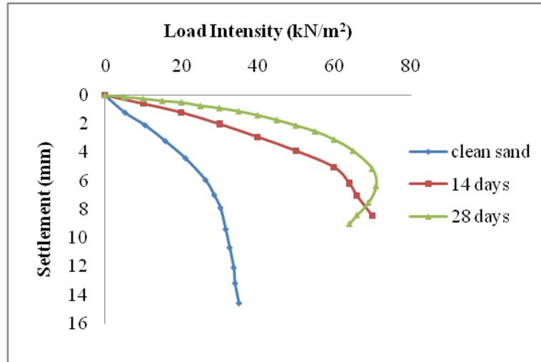
Figure 7: Load Test with Strip Footing at Distance B from Crest
