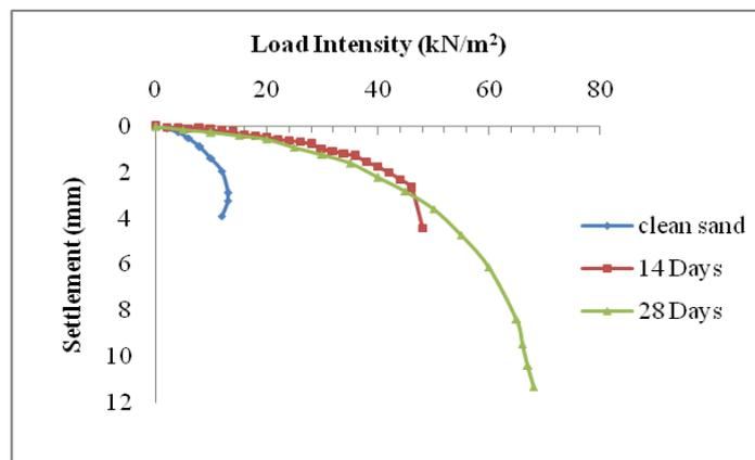
Figure 6: Load Test with Strip Footing at Crest
