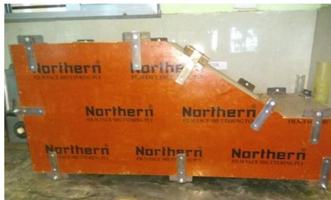
**Figure 3:** Test box of Slope of 1.5H:1V
