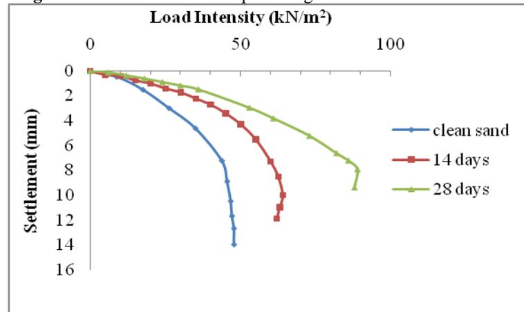
Figure 8: Load Test with Strip Footing at Distance 2B from Crest
