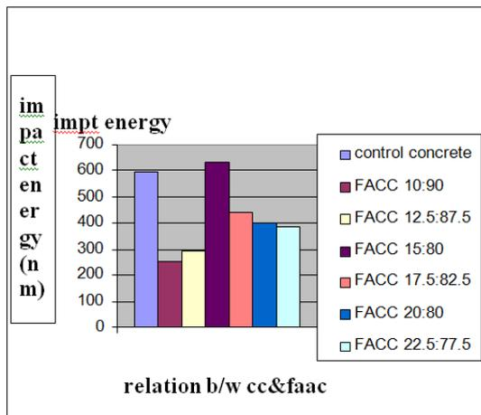
Fig. 7 cumulative impact energy of 28 days curing at initial crack
