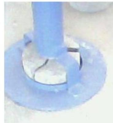
Fig.10 crack at final stage
