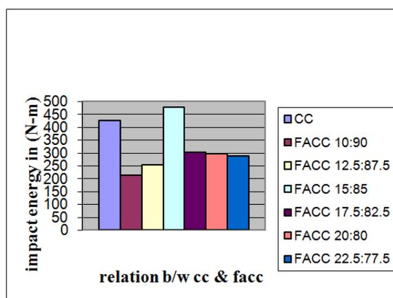
Fig. 6 cumulative impact energy of 7 days curing at final crack
