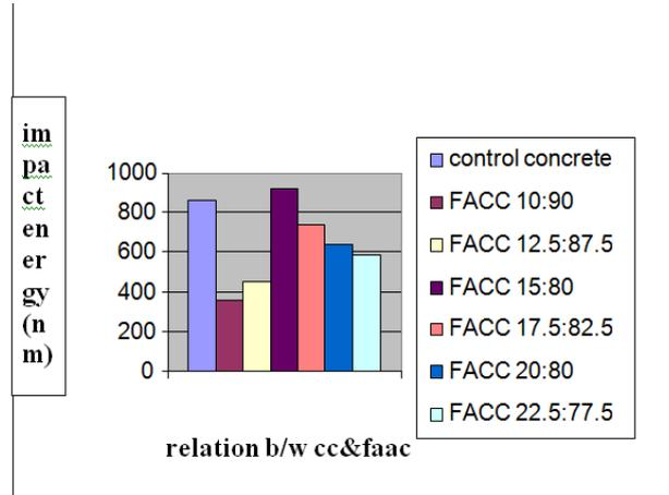
Fig. 8 cumulative impact energy of 28 days curing at final crack
