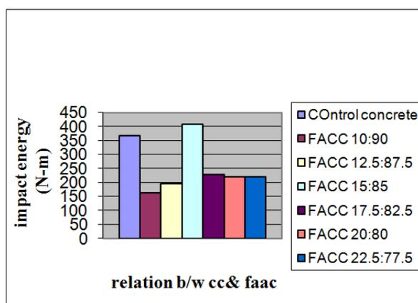
Fig. 5 cumulative impact energy of 7 days curing at initial crack
