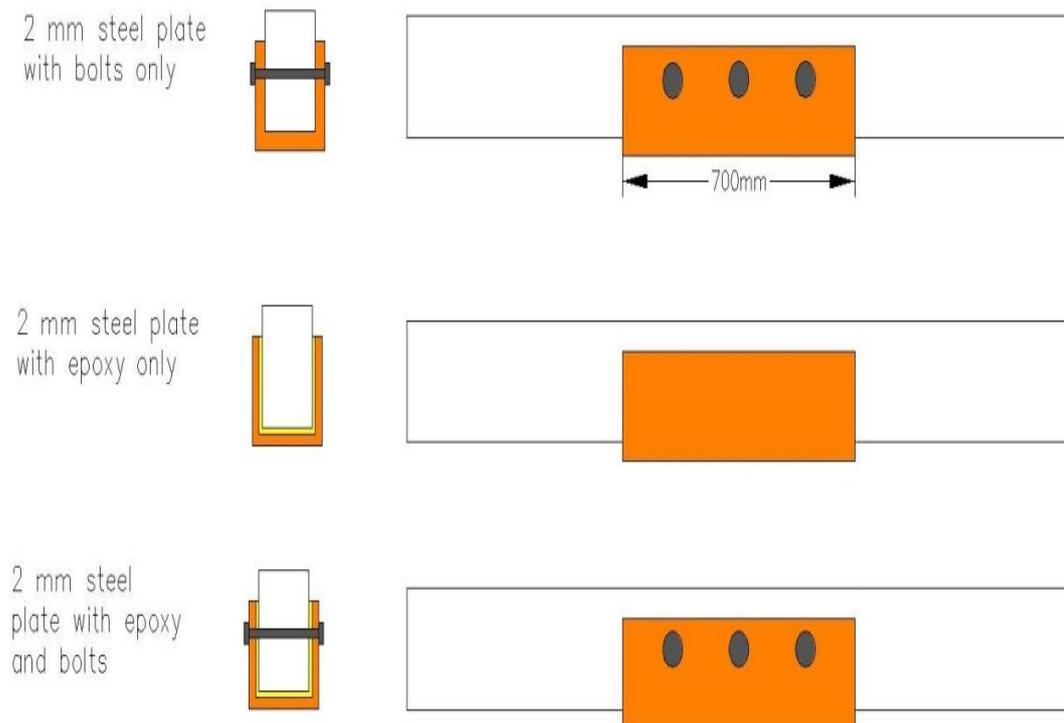
Fig. (6) Methods of fixing steel element.
