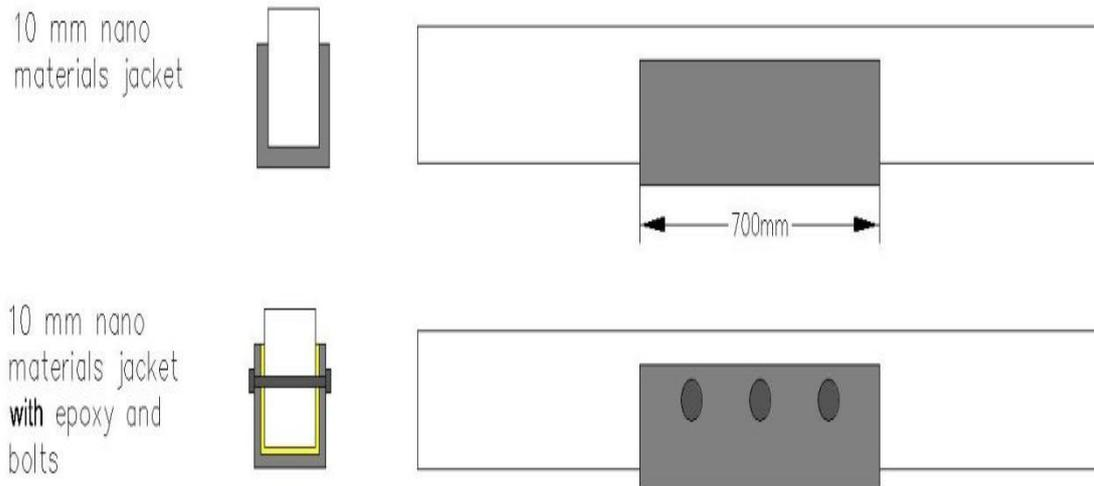
Fig. (8) methods of fixing sections made from the developed nano ferrocement.
