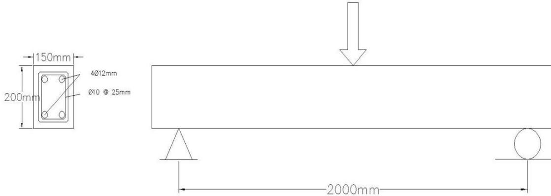
**Figure (2)** Dimensions and detailing reinforcement of the beams considered in the present investigation.
