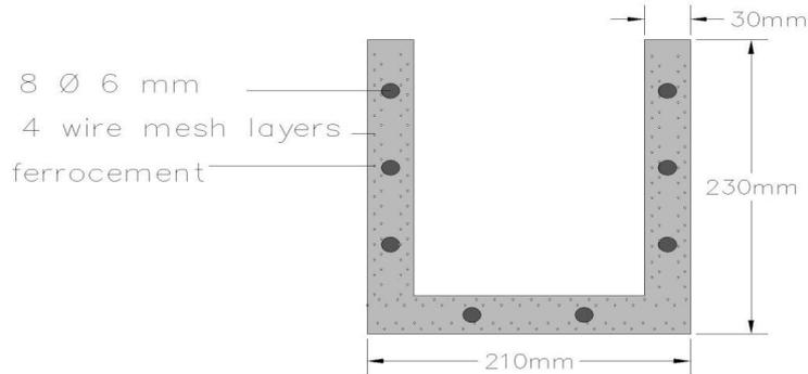
Fig. (4) Details of ferrocement cross section.
