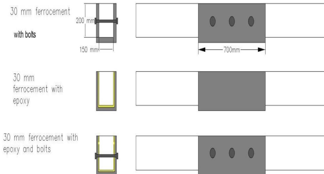
Fig. (5) Methods of fixing U ferrocement element.
