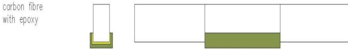
Fig. (7) Method of fixing carbon fiber layers.
