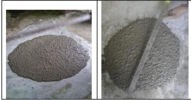
Fig.(2): Concrete Slump Flow Test
