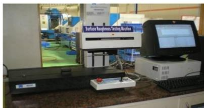
**Fig 2.** Equipment for Surface Roughness Measurement
