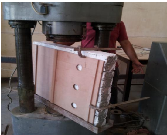
Fig- 13 Two U-steel beams for distribution load on walls
