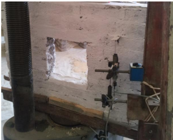
Fig-15 Wall deformations measured with LVDT
