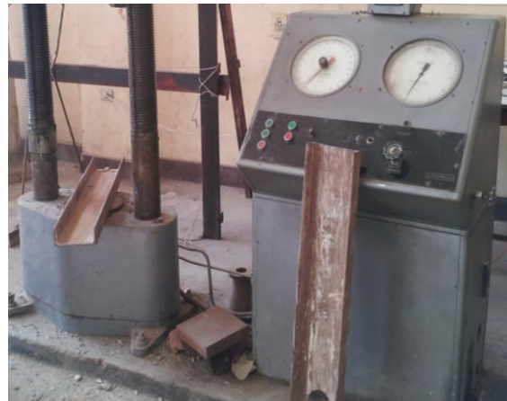
Fig- 14 Carrying wall on testing machine the by wood panels
