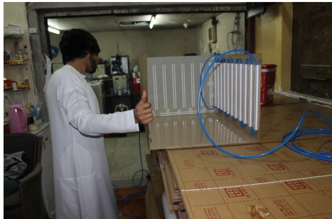
Fig.6. The rails for the plastic water tubes inside the walls.
