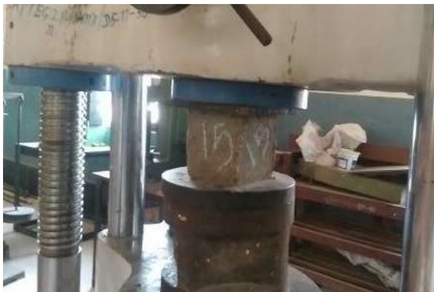
Figure 2: Compression Test Setup
