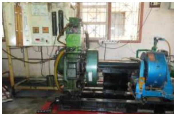
Figure 3.2. Photograph view of experimental setup (Kirloskar TV-1 Engine)
