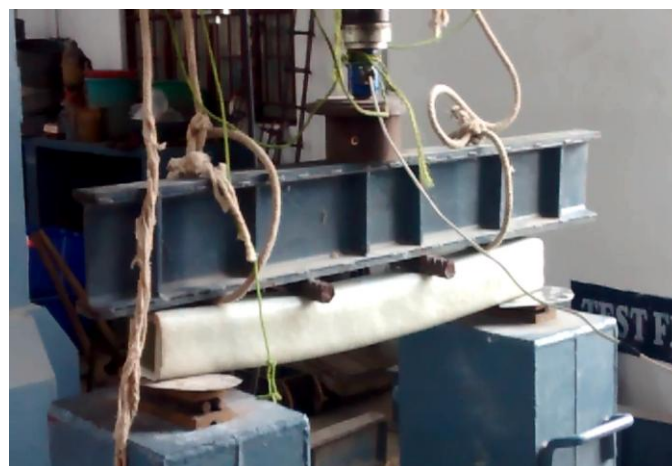
Fig-5 loading setup-deflection mode
