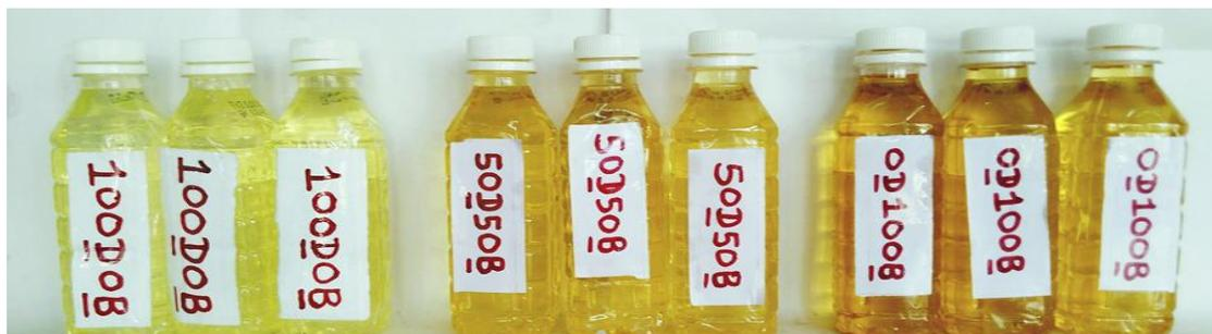
Fig 4.2.2 Diesel, Blended Fuel & Jatropha bio oil
