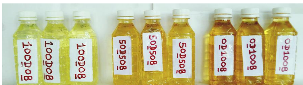
Fig 4.2.2 Diesel, Blended Fuel & Jatropha bio oil
