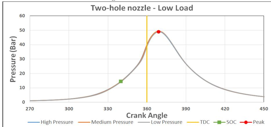
**Fig.2:** Pressure V/S Crank Angle (P-θ) graph for Low Load with two-hole nozzle
