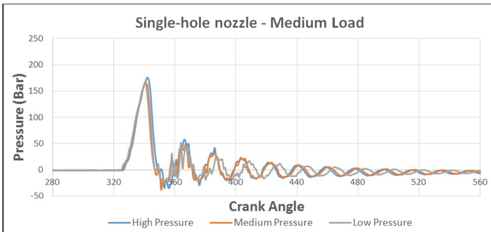
Fig.17: Fuel Line Pressure V/S Load graph for Medium Load with single-hole nozzle
