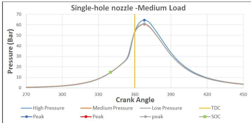
Fig.5: Pressure V/S Crank Angle (P- $\theta$ ) graph for Medium Load with single-hole nozzle
