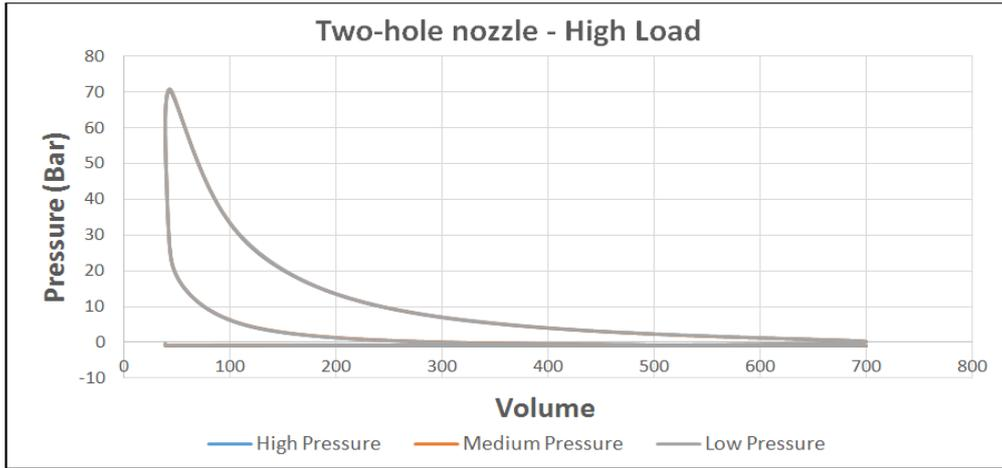
**Fig.12:** Pressure V/S Volume (P-V) graph for High Load with two-hole nozzle
