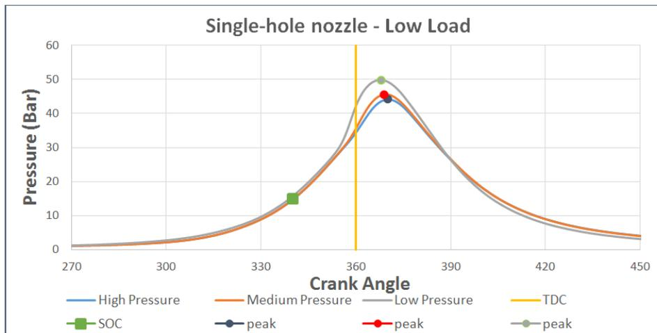
**Fig.3:** Pressure V/S Crank Angle (P-θ) graph for Low Load with single-hole nozzle
