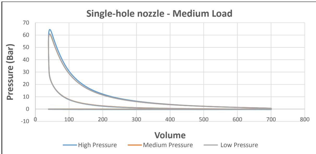
Fig.11: Pressure V/S Volume (P-V) graph for Medium Load with single-hole nozzle
