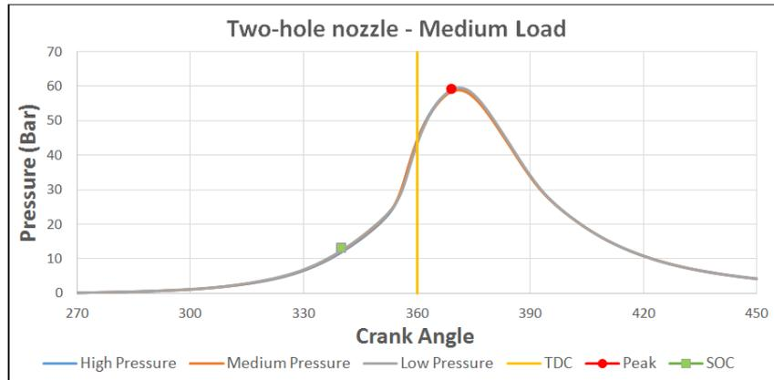
Fig.4: Pressure V/S Crank Angle (P- $\theta$ ) graph for Medium Load with two-hole nozzle
