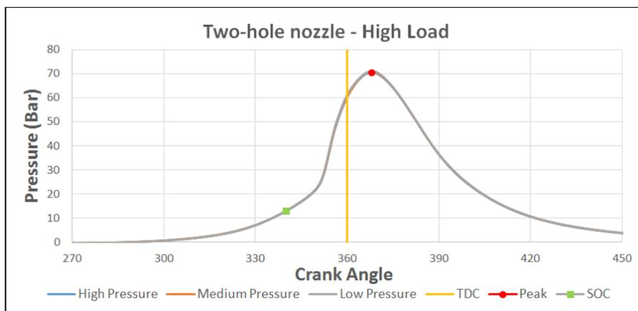
Fig.6: Pressure V/S Crank Angle (P- $\theta$ ) graph for High Load with two-hole nozzle
