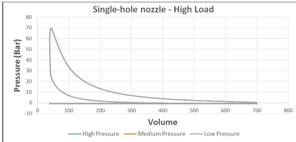
**Fig.13:** Pressure V/S Volume (P-V) graph for High Load with single-hole nozzle
