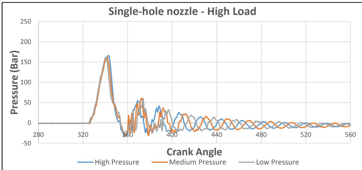
Fig.19: Fuel Line Pressure V/S Load graph for high load with Single-hole nozzle
