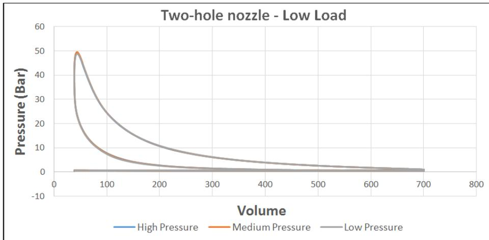
Fig.8: Pressure V/S Volume (P-V) graph for Low Load with two-hole nozzle
