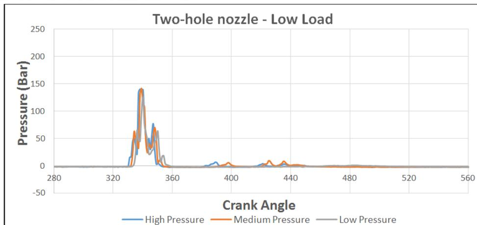
**Fig.14:** Fuel Line Pressure V/S Load graph for Low Load with two-hole nozzle
