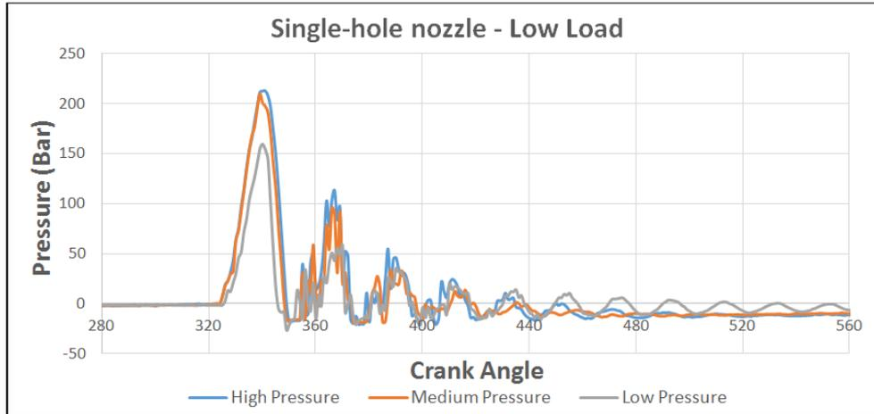
Fig.15: Fuel Line Pressure V/S Load graph for Low Load with single-hole nozzle
