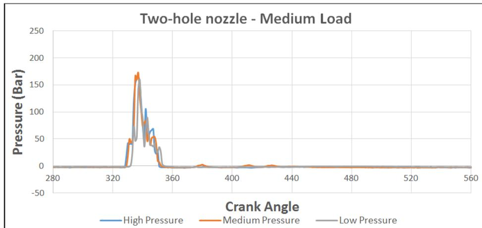
Fig.16: Fuel Line Pressure V/S Load graph for Medium Load with two-hole nozzle
