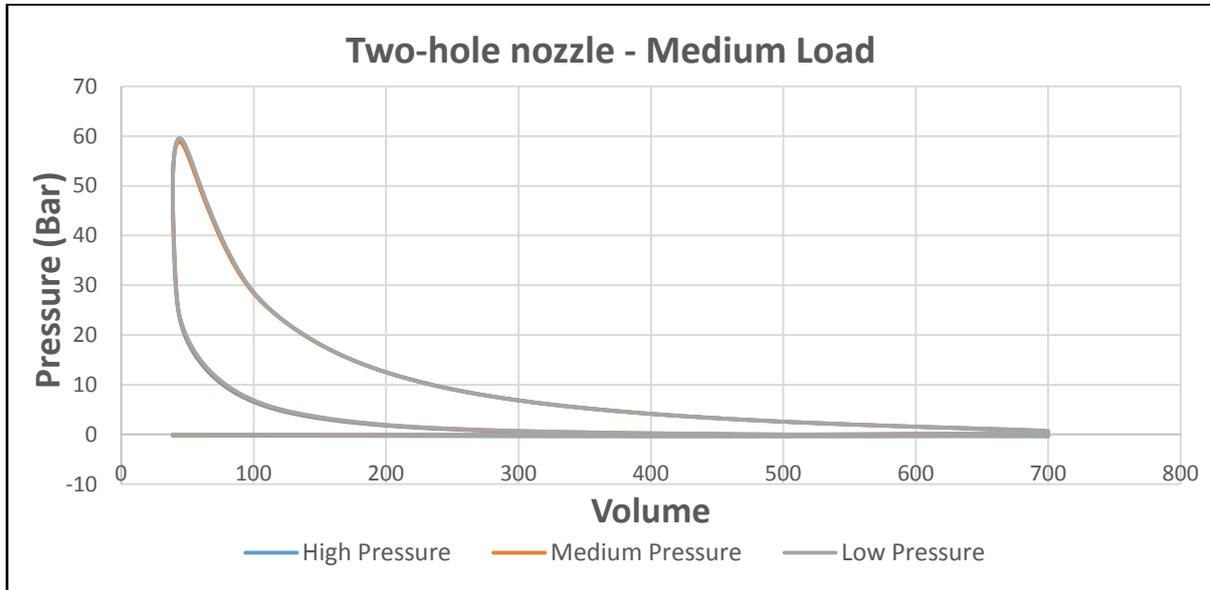
Fig.10: Pressure V/S Volume (P-V) graph for Medium Load with two-hole nozzle
