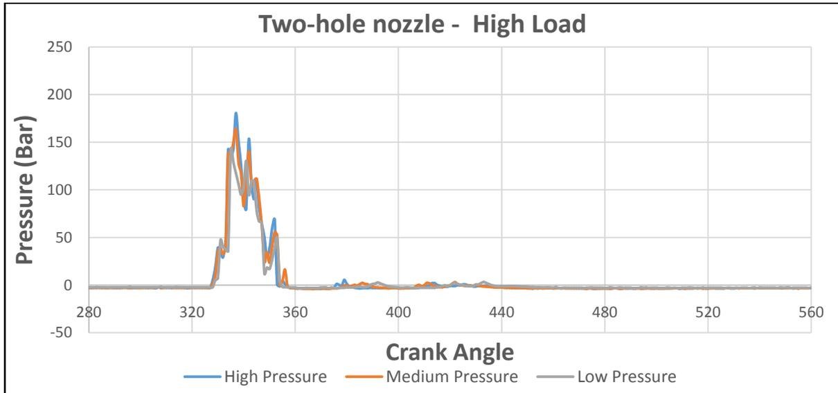
Fig.18: Fuel Line Pressure V/S Load graph for higher load with two-hole nozzle
