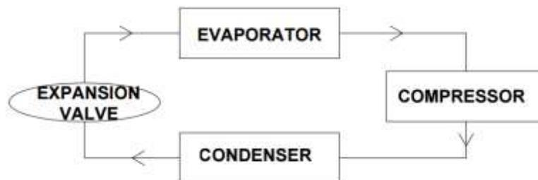
Fig. 1: Simple Vapour Compression Cycle
