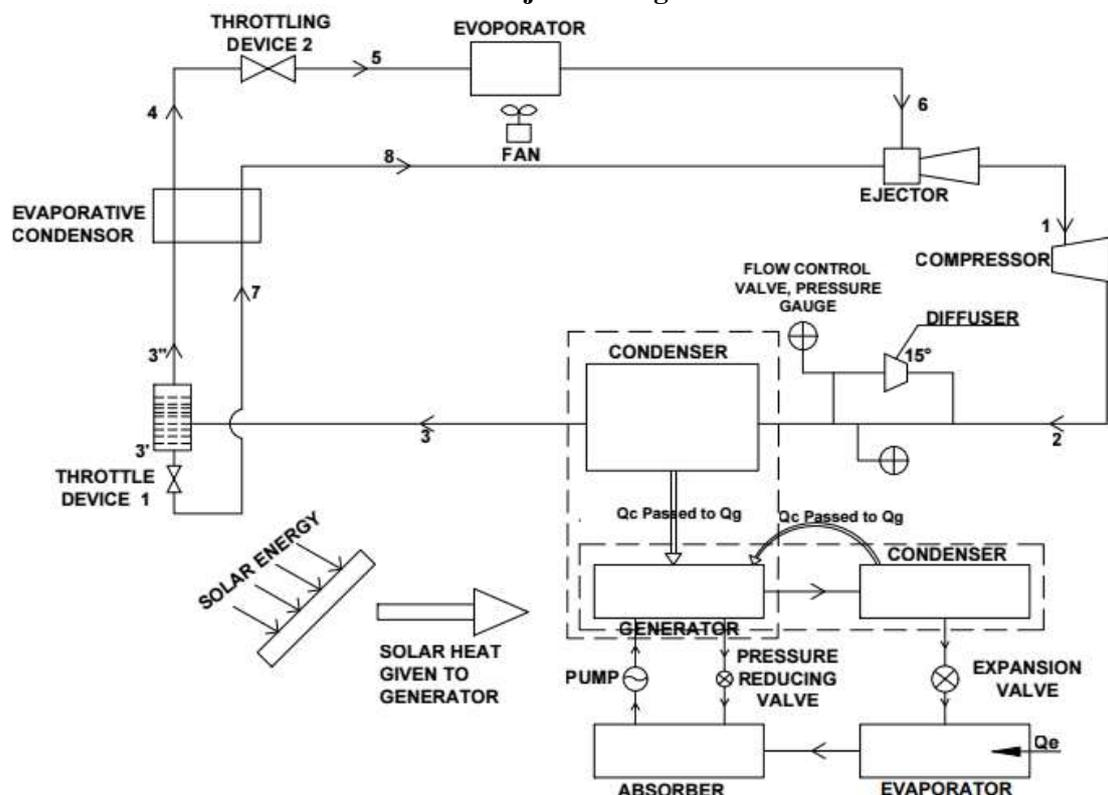
Fig. 2: Combined Vapour Compression Refrigeration System with Ejector Usage Cycle
