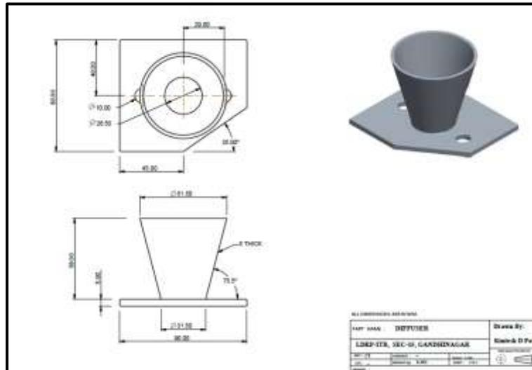
**Fig 1: 2D-3D Drawing of Diffuser A**
