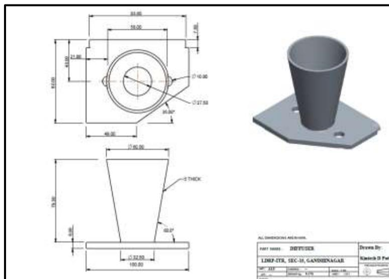
**Fig 2: 2D-3D Drawing of Diffuser B**
