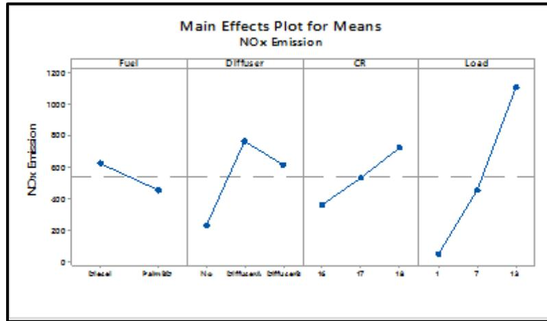
**Fig. 8:** Main Effects Plot for Means of NO<sub>x</sub> Emission
