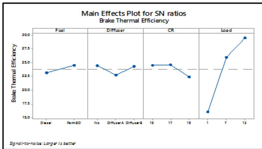
**Fig. 5:** Main Effects Plot for S/N ratios of Brake Thermal Efficiency
