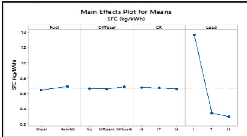
Fig. 6: Main Effects Plot for Means of Specific Fuel Consumption
