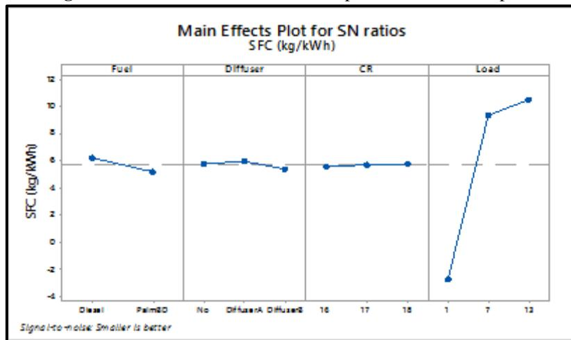
Fig. 7: Main Effects Plot for S/N ratios of Specific Fuel Consumption
