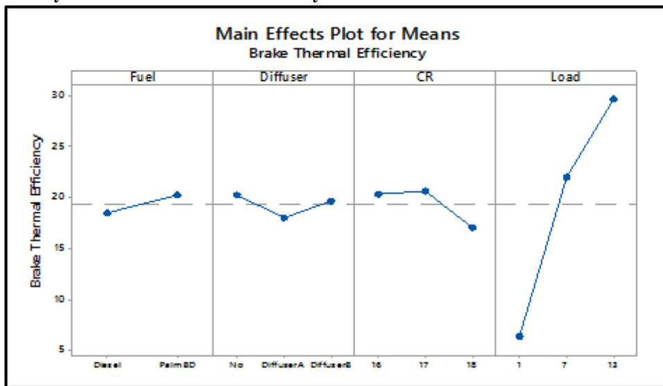
**Fig. 4:** Main Effects Plot for Means of Brake Thermal Efficiency
