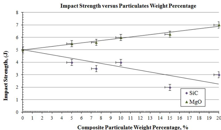
Figure 16: Effect of particulates (additives) percentage on impact strength.
