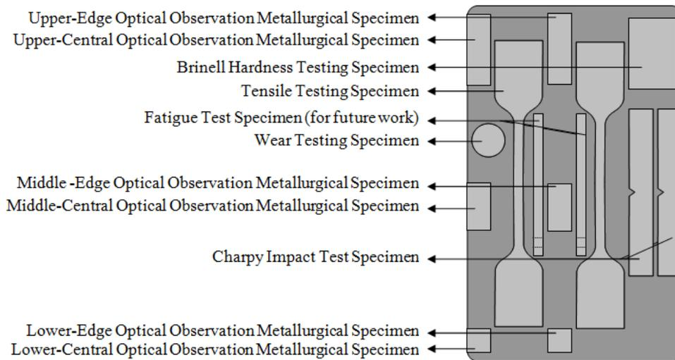
**Figure 4:** Specimens prepared for each cast
