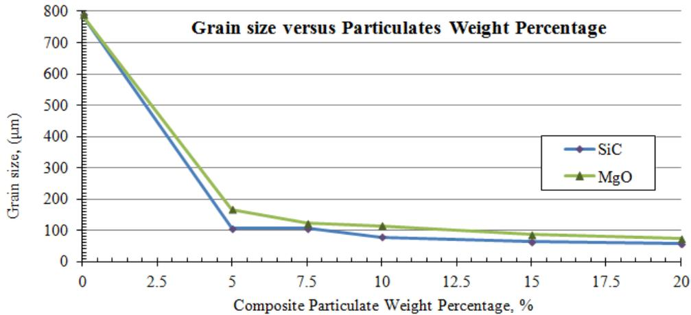
Figure 9: Effect of particulates percentage on grain size
