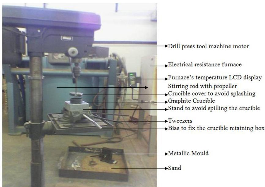
**Figure 2:** Liquid state stir mixing-casting
