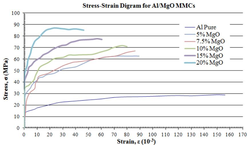
Figure 11: Stress-Strain Diagram for Al/MgO MMCs
