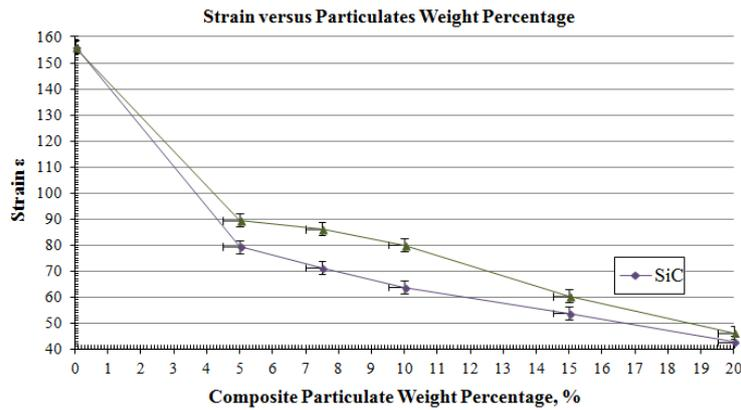
Figure 14: Effect of particulates (additives) percentage on strain.
