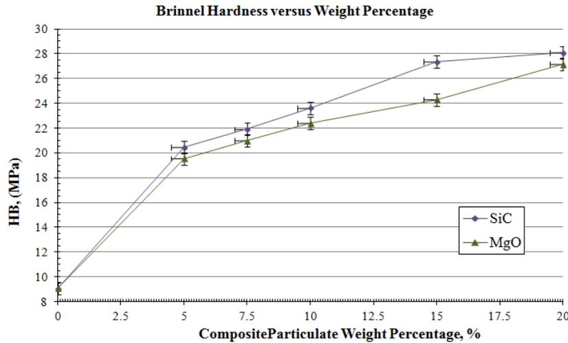
Figure 17: Effect of particulates on hardness.
