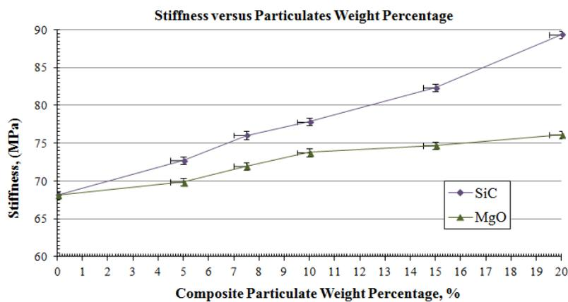
Figure 15: Effect of particulates (additives) percentage on stiffness.
