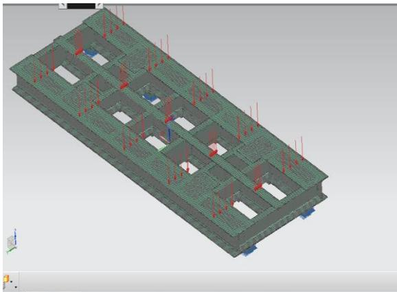
Fig. 20 Load applied downwards
