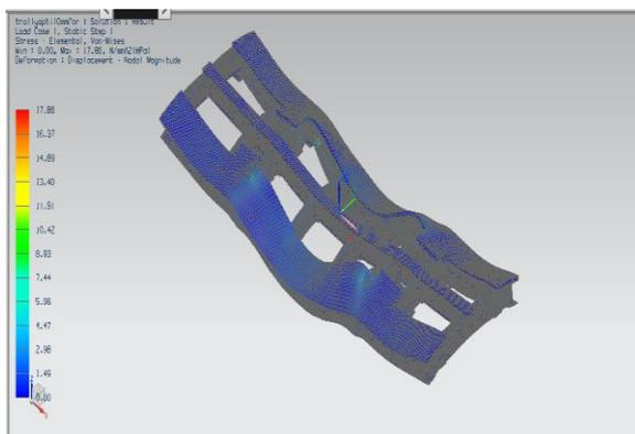
**Fig. 17** Equivalent Stress: Von-Mises: Maximum stress 17.86 MPa. Blue to red colors represents stress values from lower to higher respectively
