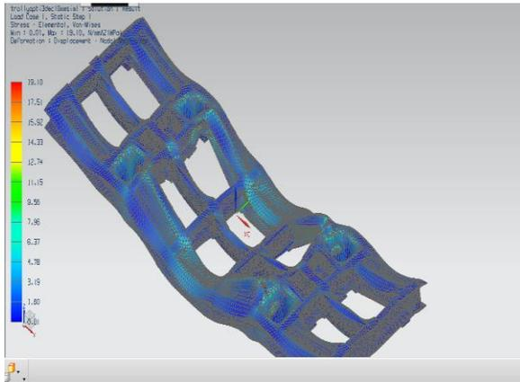
**Fig. 23** Equivalent Stress: Von-Mises: Maximum stress 19.10 MPa and Minimum stress 0.01 MPa . Blue to red colors represents stress values from lower to higher respectively
