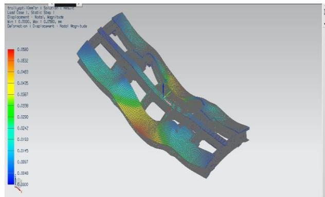
**Fig. 16** Total Deformation - Distribution of Von -Mises stresses (MPa) at trolley models. Maximum displacement 0.0580 mm and Minimum displacement 0.0000 mm .Blue to red colors represents stress values from lower to higher respectively
