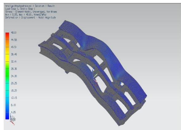
**Fig. 30** Equivalent Strain: Von-Mises: Maximum stress 48.61 MPa and Minimum stress 0.00 MPa . Blue to red colors represents stress values from lower to higher respectively
