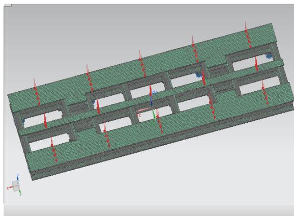
**Fig. 13** Load applies at downwards direction using solver and post-processor
