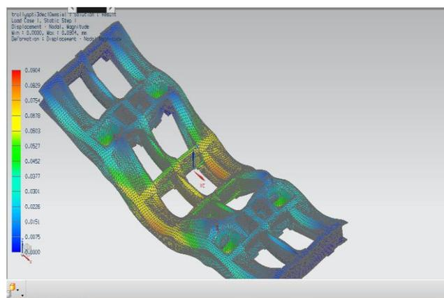
Fig. 22 Total Deformation - Distribution of Von- Mises stresses (MPa) at trolley models. Maximum displacement 0.0904 mm and Minimum displacement 0.0000 mm Blue to red colors represents stress values from lower to higher respectively
