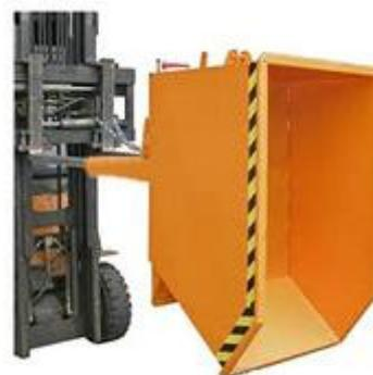
**Fig. 2** Tilting forklift trolley
