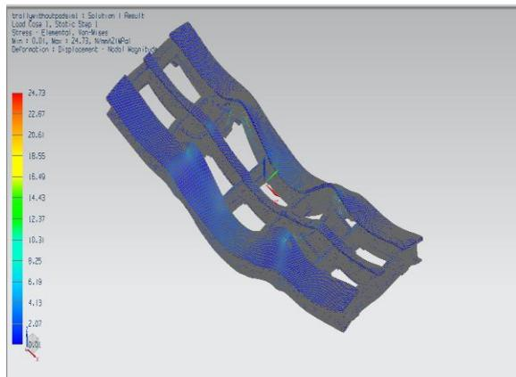
**Fig. 29** Equivalent Stress: Von-Mises: Maximum stress 24.73 MPa and Minimum stress 0.01 MPa . Blue to red colors represents stress values from lower to higher respectively
