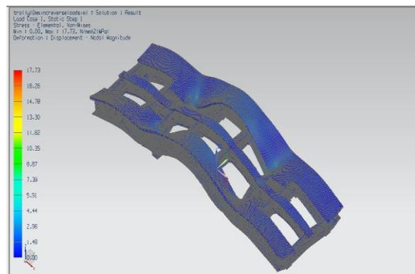
**Fig. 18** Equivalent Strain: Maximum stress 17.73 MPa and Minimum stress 0.00 MPa. Blue to red colors represents stress values from lower to higher respectively
