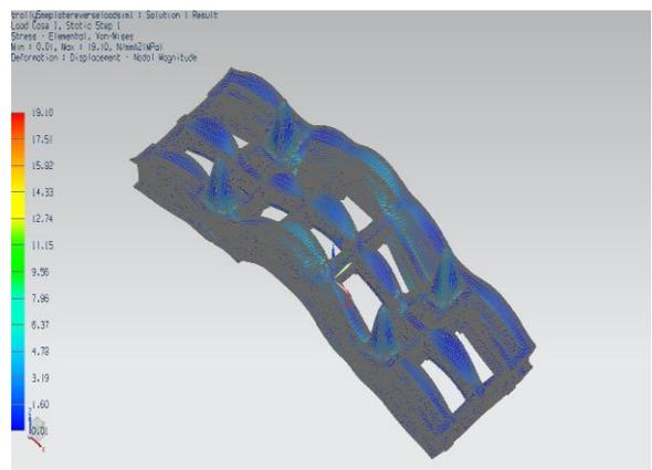
**Fig. 24** Equivalent Strain: Von-Mises: Maximum stress 19.10 MPa and Minimum stress 0.01 MPa . Blue to red colors represents stress values from lower to higher respectively
