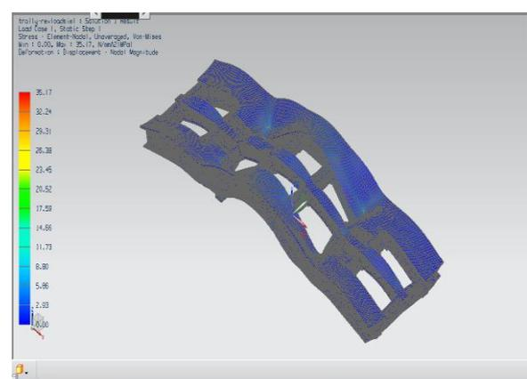
**Fig. 27** Equivalent Strain: Von-Mises: Maximum stress 35.17 MPa and Minimum stress 0.00 MPa. Blue to red colors represents stress values from lower to higher respectively
