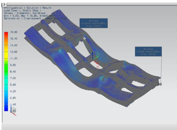
**Fig. 26** Equivalent Stress: Von-Mises: Maximum stress 16.80 MPa and Minimum stress 0.0040 MPa . Blue to red colors represents stress values from lower to higher respectively
