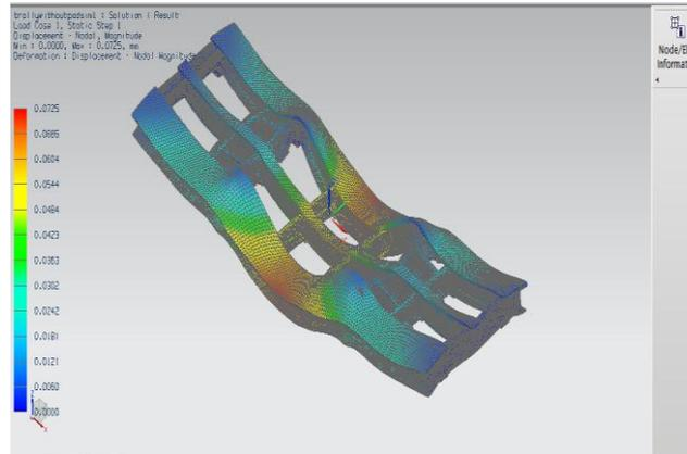
**Fig. 28** Total Deformation - Distribution of Von- Mises stresses (MPa) at trolley models. Maximum displacement 0.0725 mm and Minimum displacement 0.0000 mm Blue to red colors represents stress values from lower to higher respectively
