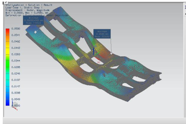
**Fig. 25** Total Deformation - Distribution of von Mises stresses (MPa) at trolley models Maximum displacement 0.0590 mm and Minimum displacement 0.0000 mm Blue to red colors represents stress values from lower to higher respectively
