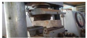
Figure 3: flexural strength test apparatus
