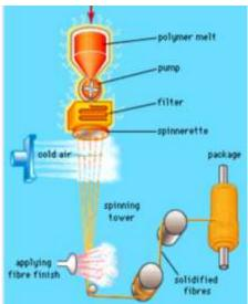
Figure 1: Melt spinning process
