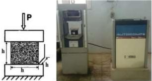
Figure 2: Compressive strngth test apparatusFlexural Strength test
