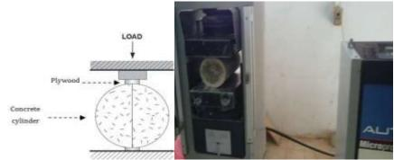
Figure 4: Splitting tensile strength test apparatus
