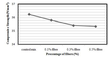
Figure 7: Relationship between compressive strength and fibre percentages after 7 days
