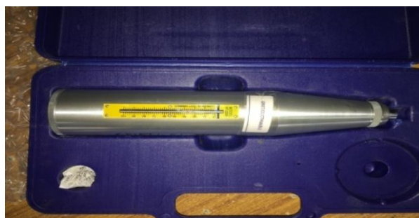
Figure 3 : Rebound hammer used
